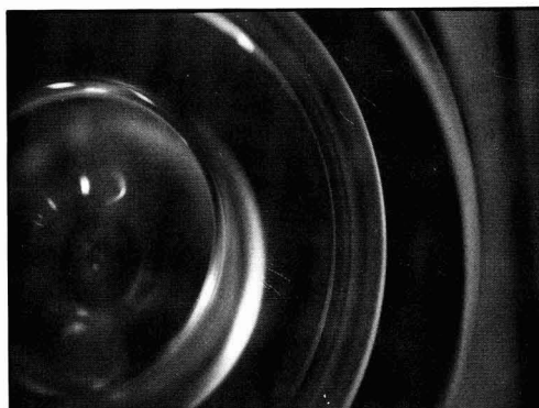
Figure 4 — Latex particle separation in the disk centrifuge for unswollen, swollen, and second generation particles
