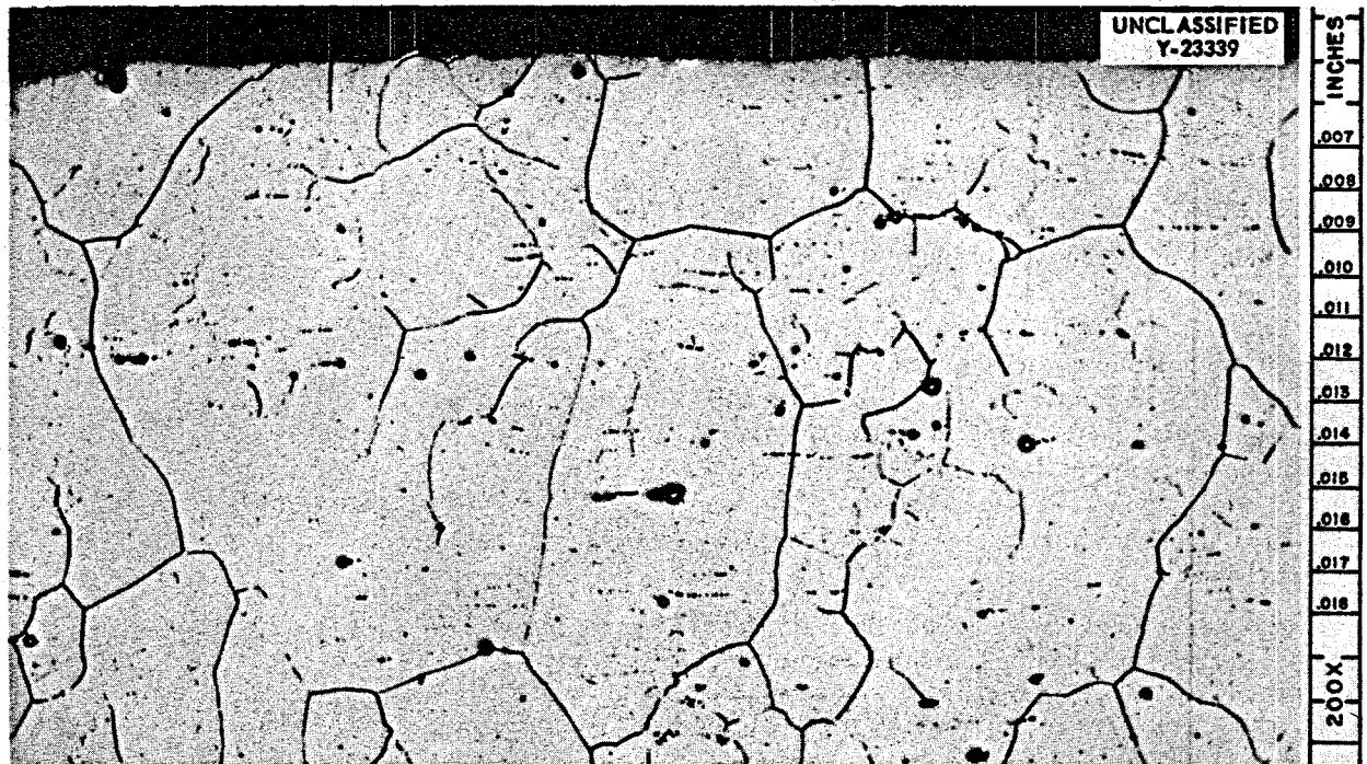
Fig. 3.6.9. Microstructure of Tube Adjacent to the Tube That Failed. No evidence of incipient failure was found. Etchant: 10% oxalic acid. 200X.
