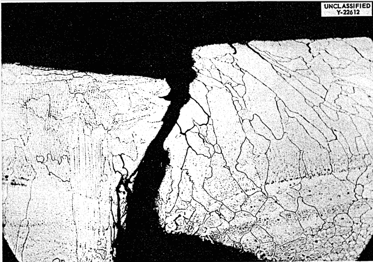
Fig. 3.3.2. Photomicrograph of Weld Fracture Shown in Fig. 3.3.1. 100X. Etchant: electrolytic oxalic acid.
