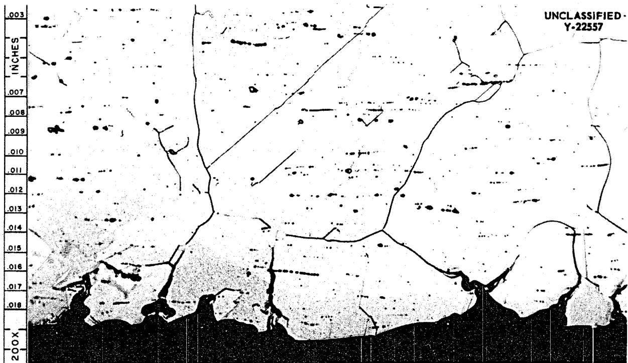
Fig. 3.6.16. NaK-Side Surface of Tube Shown in Fig. 3.6.15. Etchant: 10% oxalic acid. 200X.
