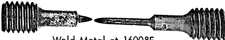
Weld Metal at 1600°F
