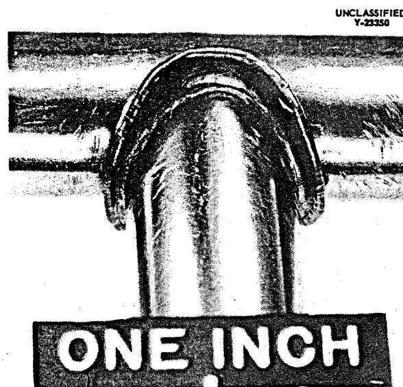
Fig. 3.4.9. Niobium Tubing Saddle Weld.
