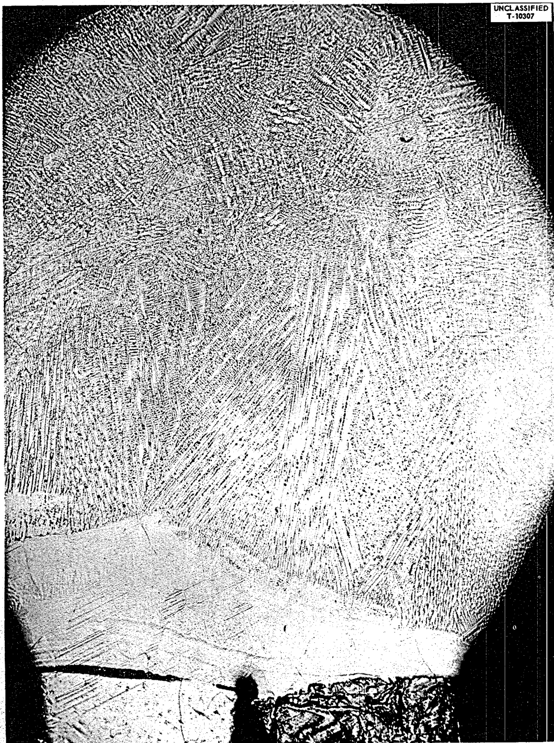
Fig. 1.3.20. Cross Section of Heliarc-Welded Junction of Inconel-Coated Chromel-Alumel Thermocouple Wires. Chromium oxide deposits may be seen in the Chromel wire.
