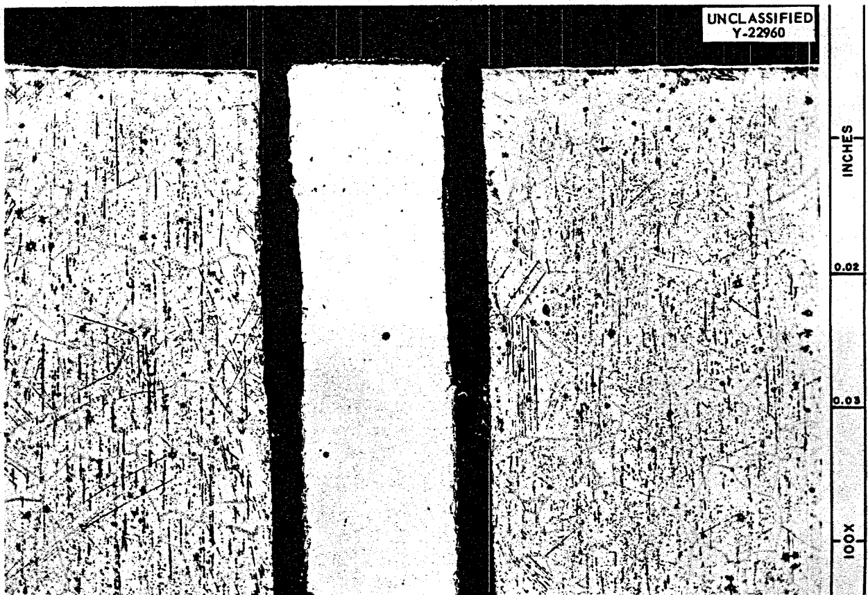
Fig. 1.7.7. Photomicrograph of End of "Gunbarrel" Thermocouple After 300 hr of Exposure to Static NaF-ZrF 4 -UF 4 (50-46-4 mole %) at 1200°F. Note the absence of the nickel plate between the end of the central nickel wire and the Inconel on either side. (Secret with exception)
