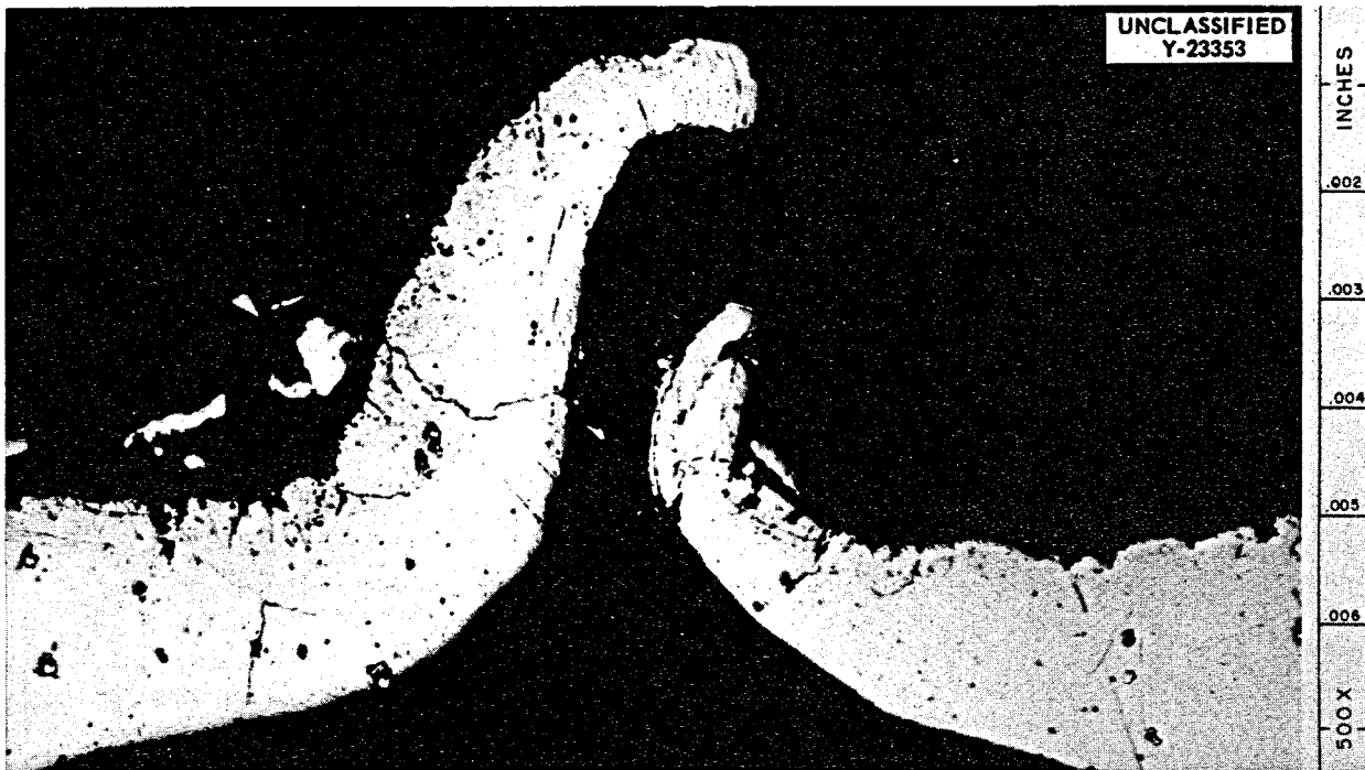
Fig. 3.6.7. Higher Magnification of Fig. 3.6.6. No evidence of incipient failure may be seen. Etchant: 10% oxalic acid. 500X.
