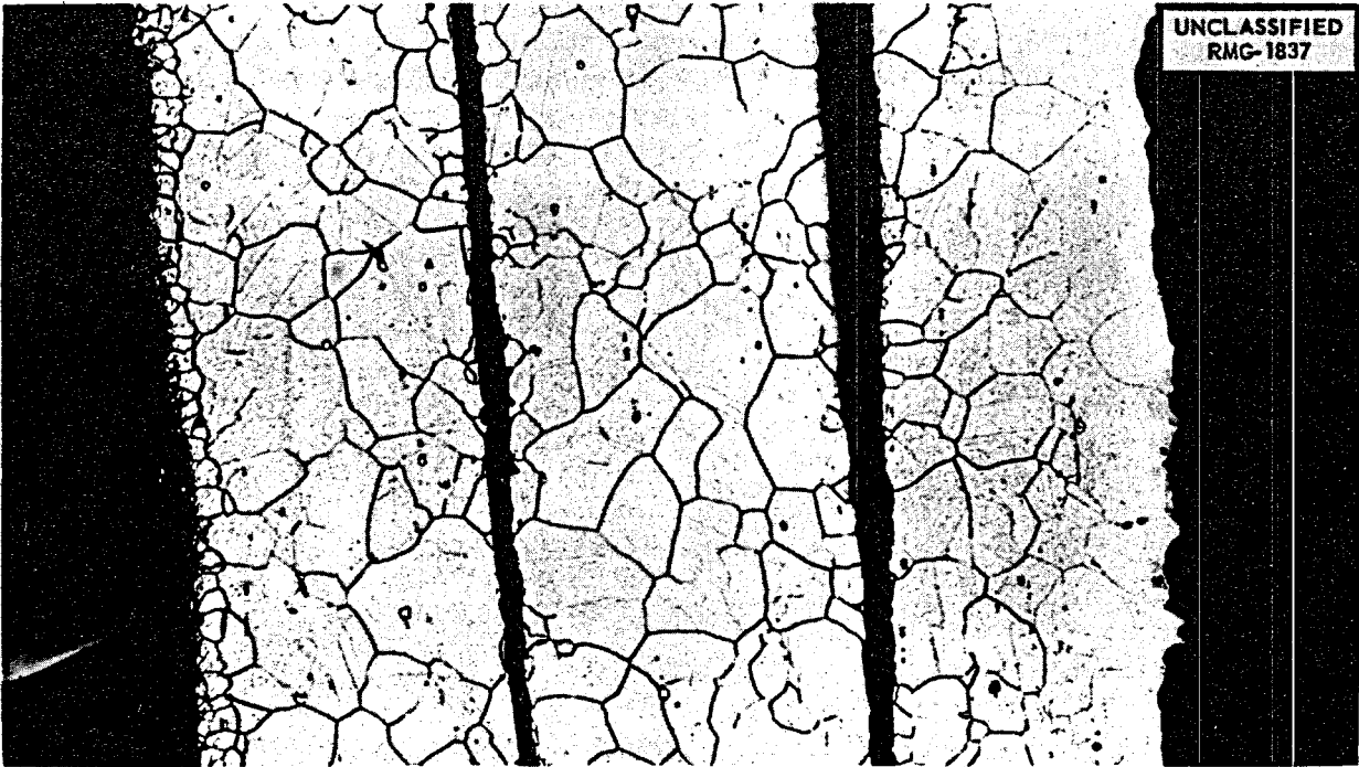
Fig. 4.1.21. Section of Specimen S6 Taken from the Bottom Bellows of Sodium Valve U-23. Etched. 250X. (Secret with caption)
