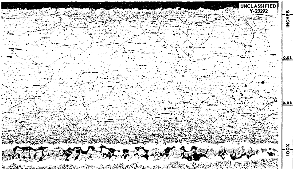
Fig. 3.6.22. NaK Corrosion in Tube Wall Adjacent to Weld Shown in Fig. 3.6.19. Etchant: electrolytic oxalic acid. 100X.
