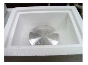
**Fig. 3** Aluminum disc, approximately 125 mm in diameter ×15 mm, on dry ice inside a Styrofoam shipping carton.
