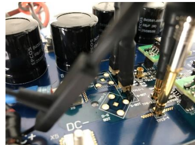
Paralleling SMD resistor shunt + MMCX
