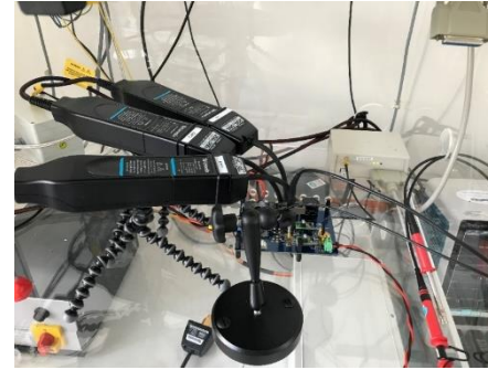
V_{gs} measure: Use MMCX connector OR optical isolated probe (very expensive)
