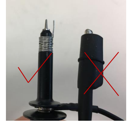
Use wire wound connection instead of alligator clip
