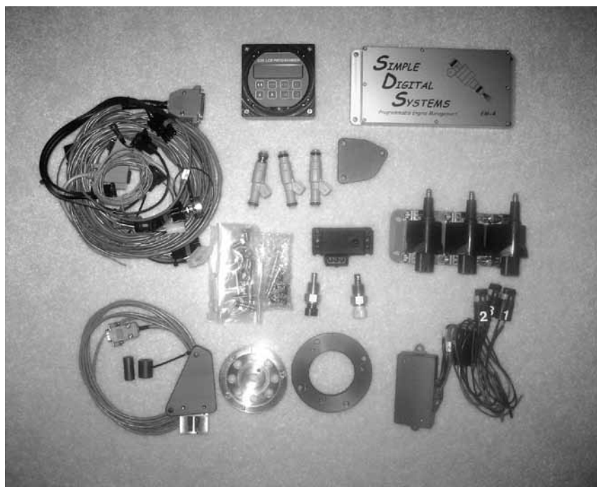
Simple Digital Systems G10 kit plus my own camshaft adapter
