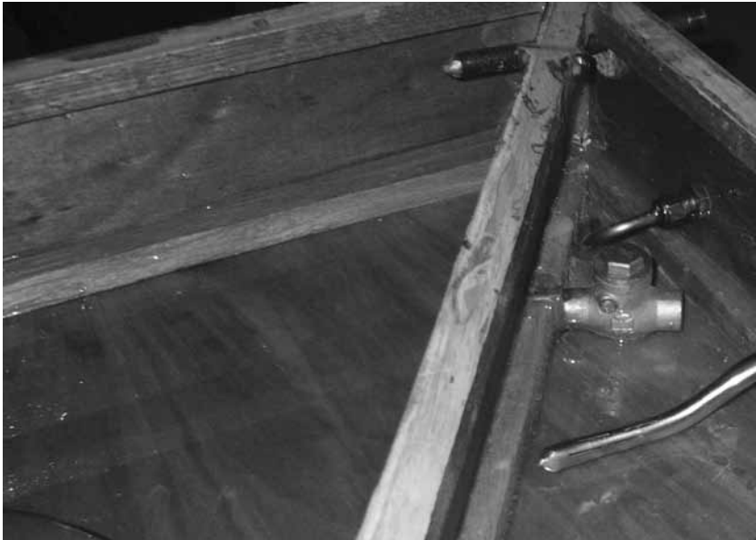
Above: The picture of the uncovered wooden gas tank shows most of the hardware involved. From the top; fuel filler, fuel drain, one of several check valves, fuel out to engine – this is the rear one, mechanical fuel gauge, and ground wire. Other stuff not shown here include pressure relief tubes between the sections and overfill drains.
