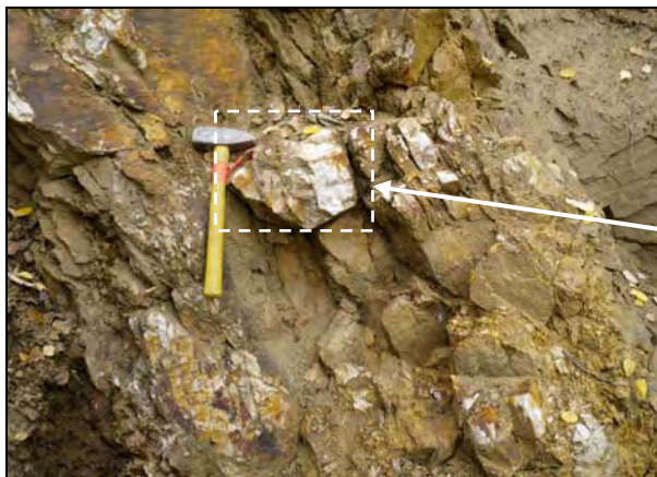
Photos M2. Detailed character and relative location of anomalous gold-bearing quartz vein samples and altered wall rock collected from the Alphonse vein central/main trench showing.
