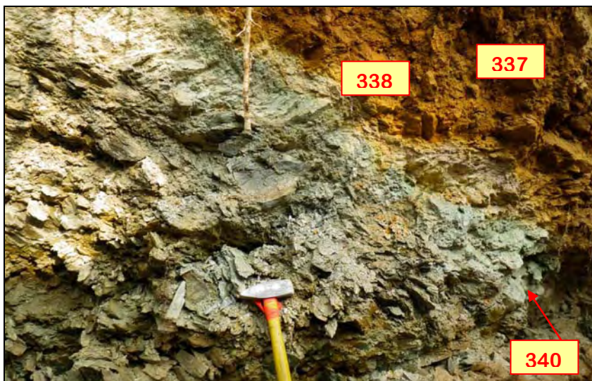
Photos M9. Alteration in mafic and ultramafic rocks at tectonized contact in pit SE of Mt. Leotta. Sample locations indicated as labeled. Assay results provided in Table 8.
