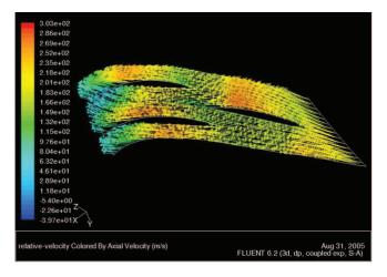
Figure 4. Vectors of relative velocity in a cylindrical layer of the tandembladed impeller (a previous calculation) [7]
