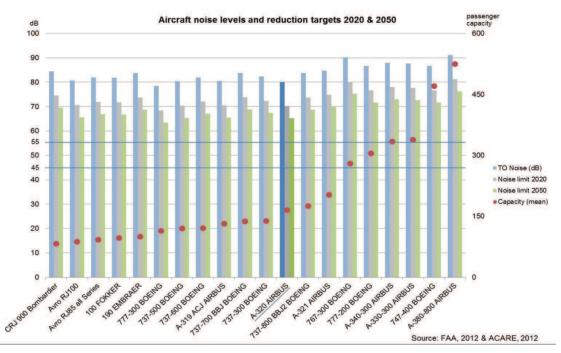
Figure 2. aircraft types operating in Europe, aircrafts' capacities and current take-off noise levels[6]
