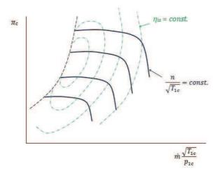
Figure 5. A typical compressor map
