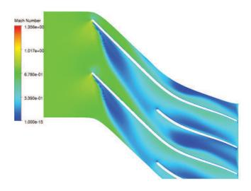
Figure 9. Relative velocity Mach number distribution inside the impeller at 95% span
