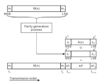
Figure 1. Downlink parity encoding process for DF 0, 4, 5, 16, 20, and 21 replies [2]
