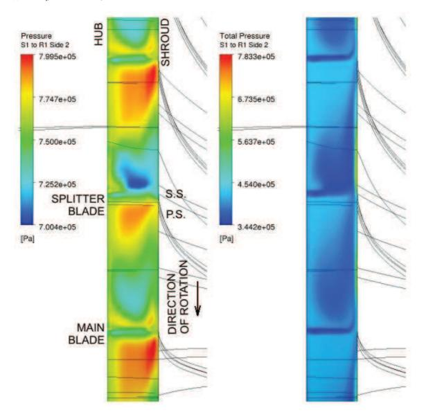
Figure 10. Pressure distributions at impeller exit. Left, static pressure. Right, total pressure.
