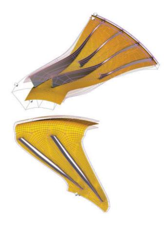
Figure 7. Above, impeller computational mesh. Below, diffuser mesh
