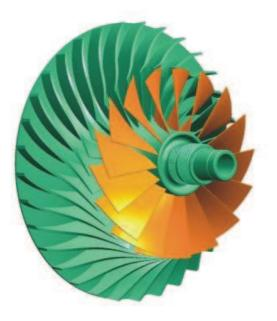
Figure 3. A study of a tandem-bladed impeller [7]
