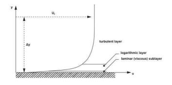
Figure 6. A scheme of near-wall flow layers [2]
