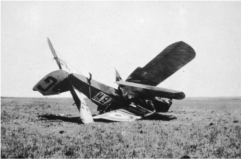
Figure 16 Second crash of plane at High River. On May 31, 1921, May F/O A. Carter, with crewman Beattie was landing G-CYBW at High River and, on the approach, the pilot was side slipping off excess height, but failed to level out before striking the ground. The left wing collapsed and the aircraft broke up on contact. The pilot and crewman were seriously injured and the D.H.4 was damaged beyond repair (source: Glenbow Museum NA-2097-56)
