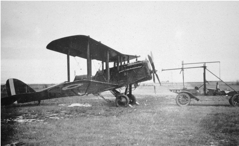
Figure 7 De Havilland 4 Huck Starter at High River Air station ca. 1926. Automatic starter built on chassis of Model T Ford car (source: Glenbow Museum NA-2097-25 )
