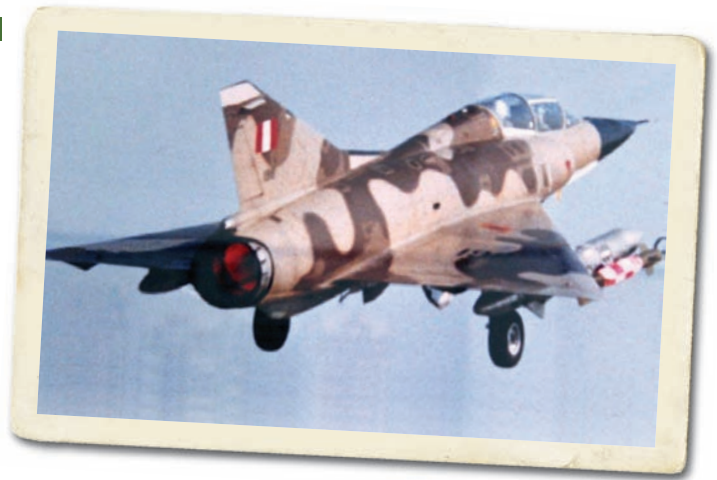
Mirage 5DP2 FAP 198 testing French SAMP EU2 500 pound laser-guided bombs. Archive Sergio de la Puente
