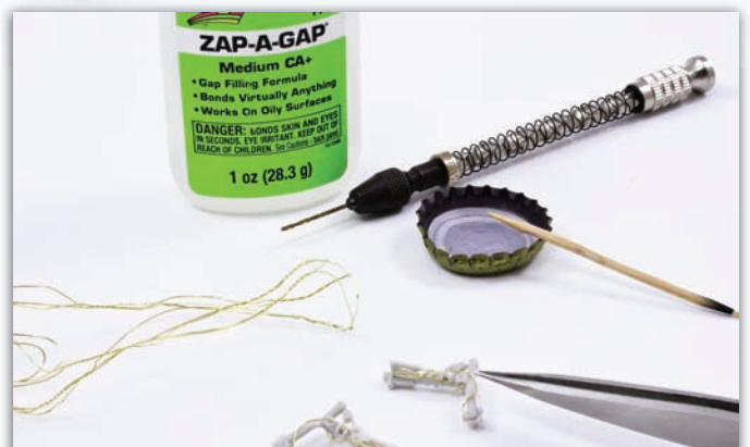
Brake lines are added using fine wire, using superglue to fix them into holes pre-drilled with a pin vice.
