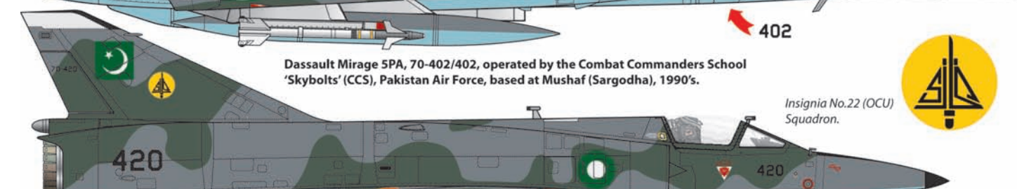
Dassault Mirage 5PA, 70-420/420, operated by No.22 (OCU) Squadron, Pakistan Air Force, based at Masroor, 1990's. The devices atop the dorsal antenna and windscreen are forwards and rearwards-facing RWR's.
