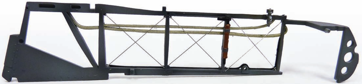
The left fuselage frame detail is almost completely replicated after the addition of the bracing wires, added using rolled steel wire.
