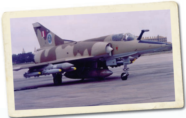
Mirage 5P3 FAP 110 loaded with eight 250 pound Snakeye bombs. Archive Lewis Mejía
