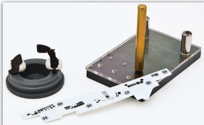
Using a round punch-&-die set, some leftover decals were "raided" in order to add faces to the instrument panel dials.
