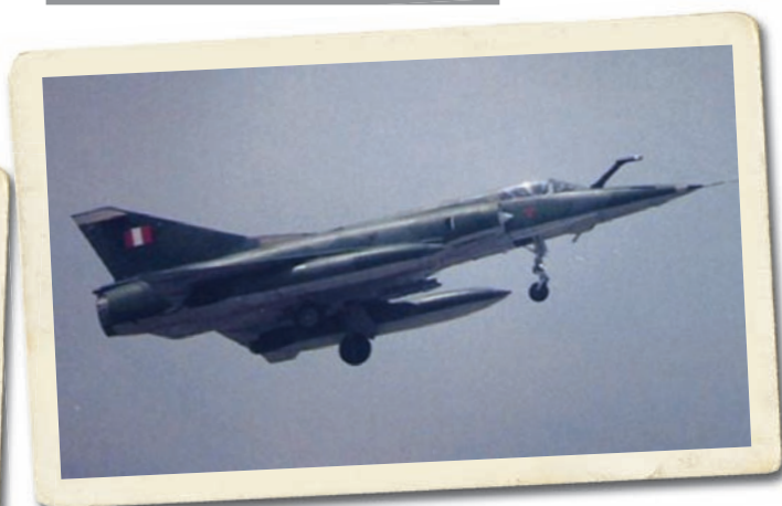
A Peruvian Mirage 5P sporting two-tone green camouflage, with refuelling probe and Laser telemeter, installed by Dassault from 1982 on all of the fleet. Archive Lewis Mejía
