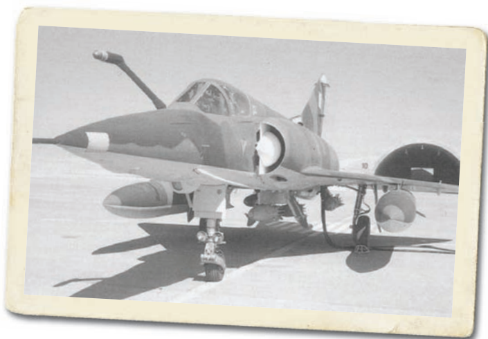
A Modernized Mirage 5P with four 500 pound Snakeye bombs. Archive Amaru Tincopa
