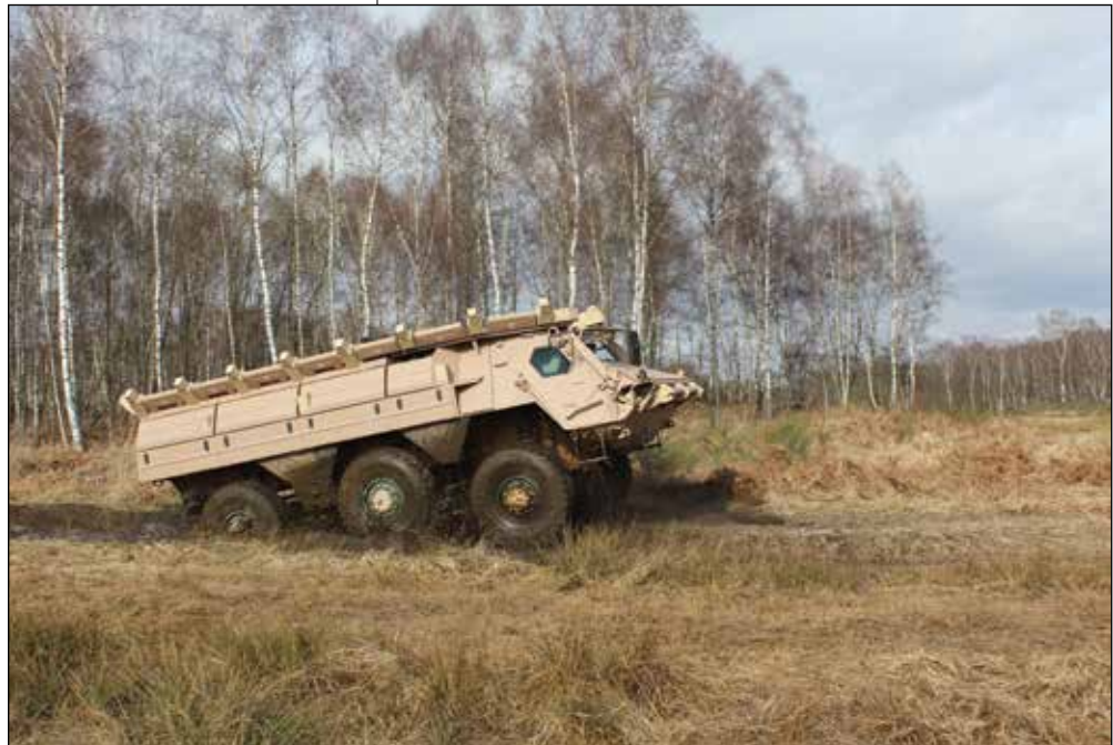
A RMMV Fuchs 1 A8 IFV equipped with ADS HAT ~ A full rocket and missile Active Defence System.
