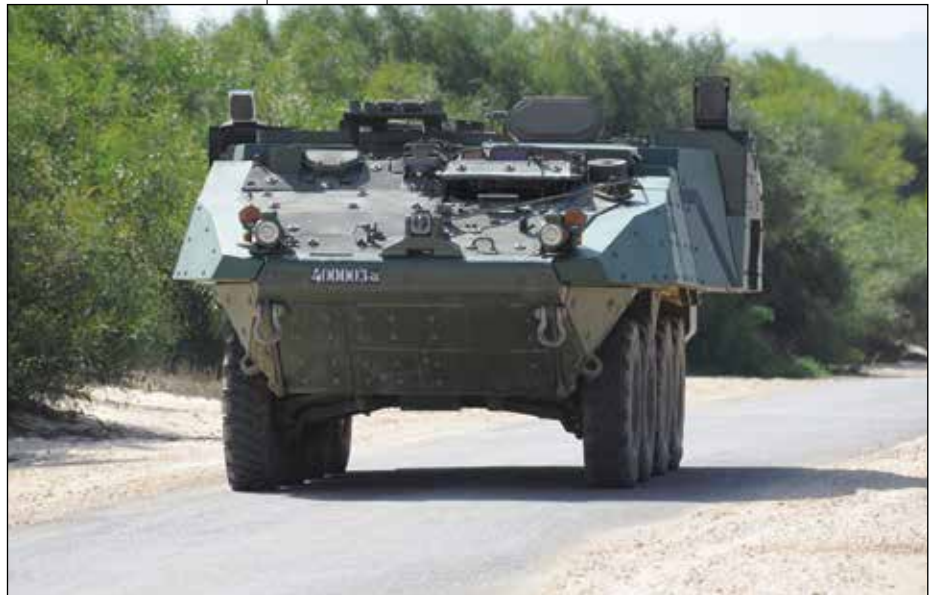
Trophy mounted upon and successfully integrated with a General Dynamics (Land) Stryker Infantry Fighting Vehicle (IFV). The Stryker is derived from the Canadian LAV III IFV.
