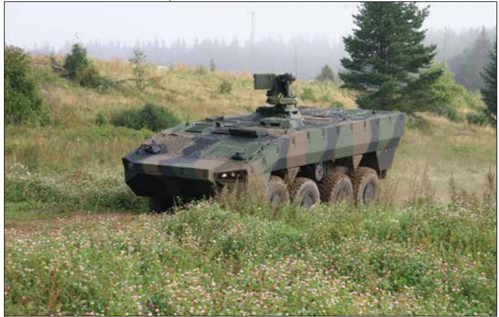
A Patria AMV (8x8) equipped with ADS HAT ~ A full rocket and missile Active Defence System.
