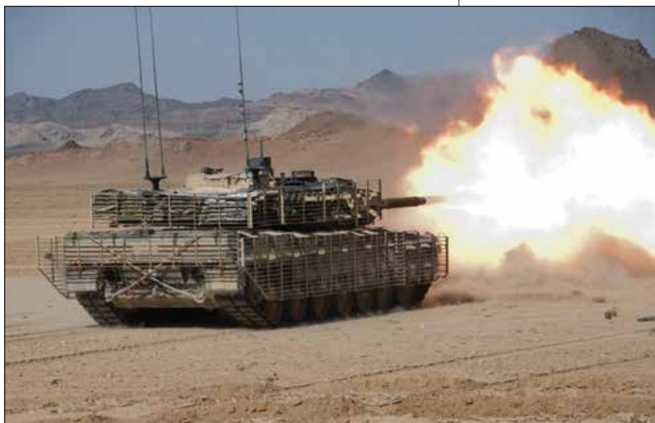
A Leopard 2 tank firing to adjust its 120 mm gun in the Panjwa'i district of Afghanistan, 14 February 2008.
