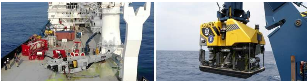
Navy MH-60S helicopter lies upside down on the deck of a contracted salvage vessel (left) after recovery by Navy CURV 21 (right), a 6,400-pound remotely operated vehicle used for deep ocean salvage
