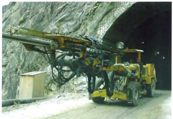
Jumbo Boomer-353 is used for excavation of Road tunnels
