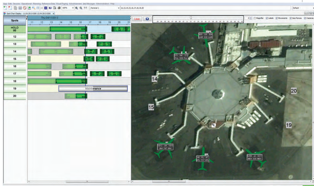
Real-time data about gate utilization enhances ramp safety.
