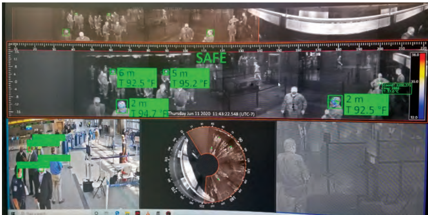
Thermal imaging allows LAX to conduct wide-scale temperature checks as passengers and other guests enter the terminal.
