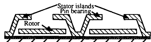
Figure 1(b). Released micromotor structure
