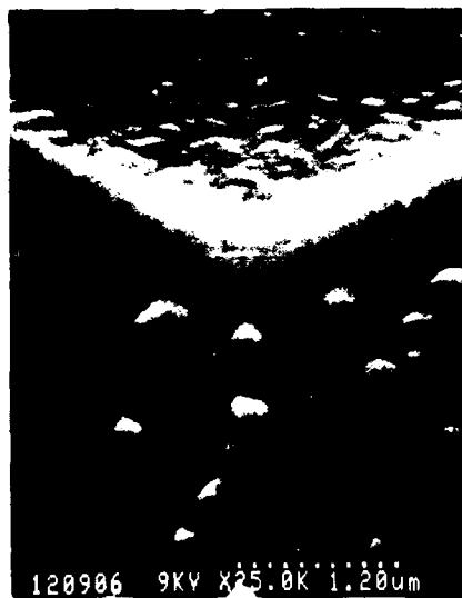
Figure 3. Silicate dust from VHF-etched nitride
