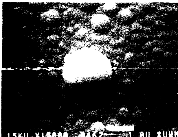
Figure 2. Protrusion (~1 \mu\text{m} high) in a 2 \mu\text{m} thick polysilicon film. The rough texture around the nodule finds its origin in the underlying silicon nitride film.
