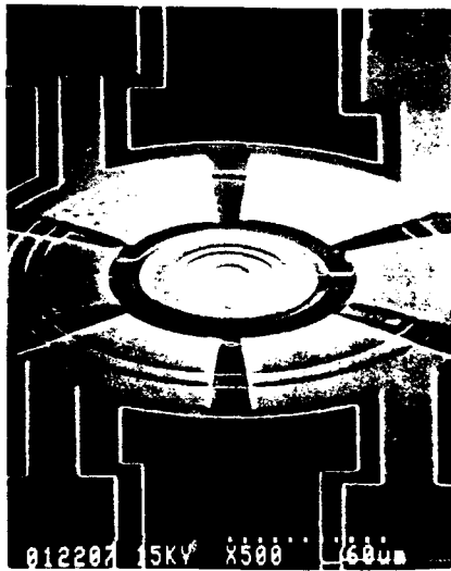
Figure 6. Poly-Si micromotor structure released with LHF
