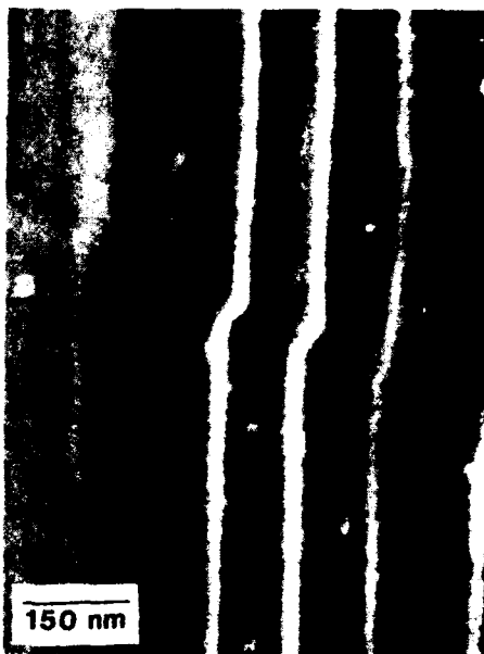
Figure 2. HRSEM image of a 50 nm single kink with two sharp, well defined boundaries. \alpha = 34.5^\circ , \beta = 21.5^\circ
