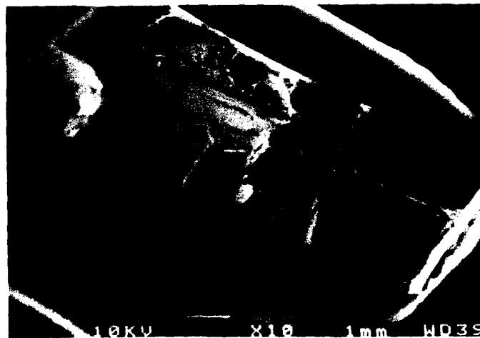
figure 4 SEM fractography of a sample under discontinuous fatigue test (DFT)
