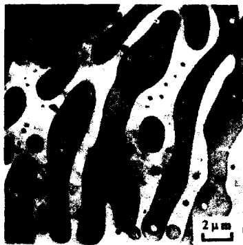
Figure 4 a.) Bi-continuous structure of PBT/PC blend
