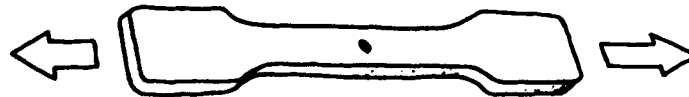
Figure 1 Used tensile specimen with central hole. Dimensions: effective length: 100 mm, width: 10 mm, thickness 4 mm, hole diameter 2 mm.
