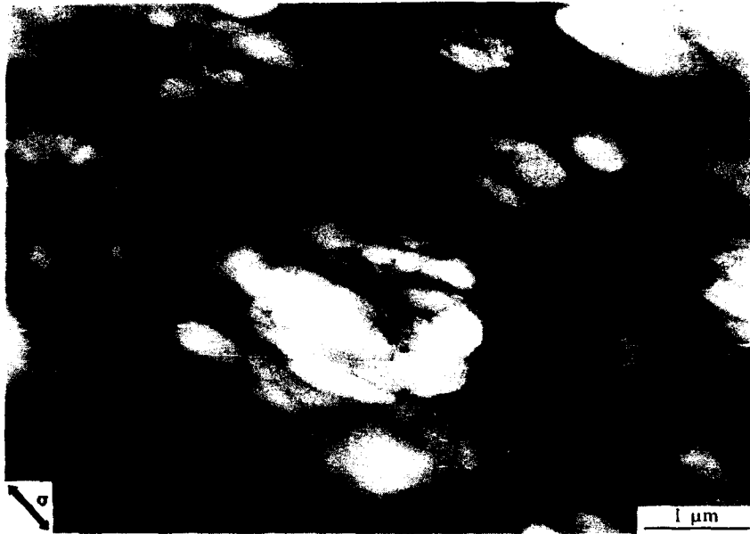
Figure 2 Void formation inside the rubber particles of impact polyamide, HVEM
