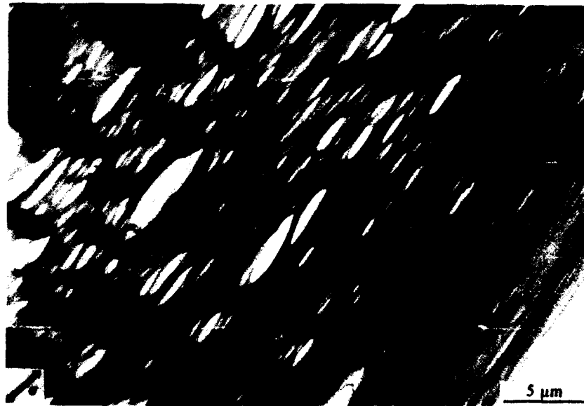
Figure 1 Deformation structure of high impact polypropylene, HVEM
