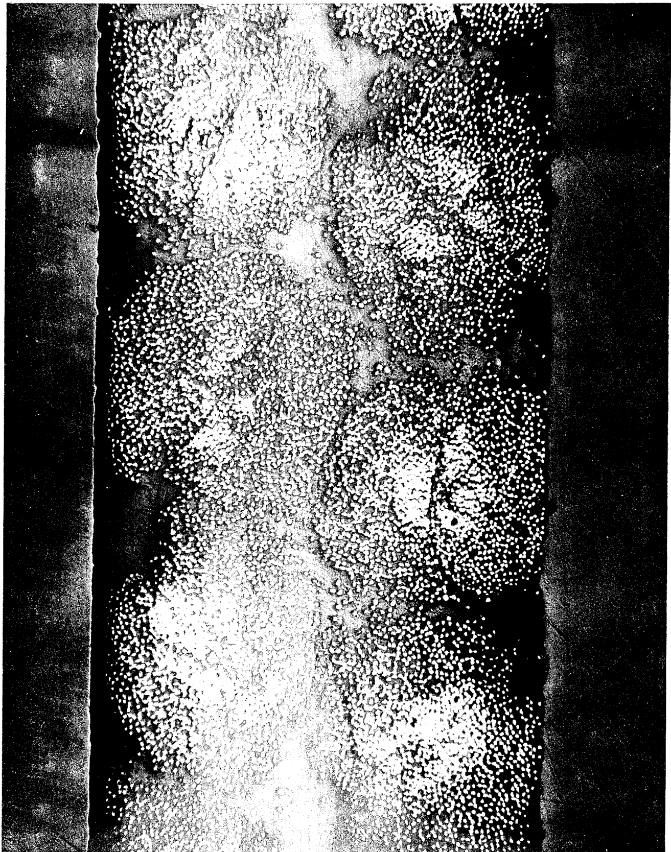
Fig. 30 - (100X) HMG-50/epoxy specimen after 13.04 \times 10^4 amperes per \text{cm}^2 of filament crest current injection--no damage
