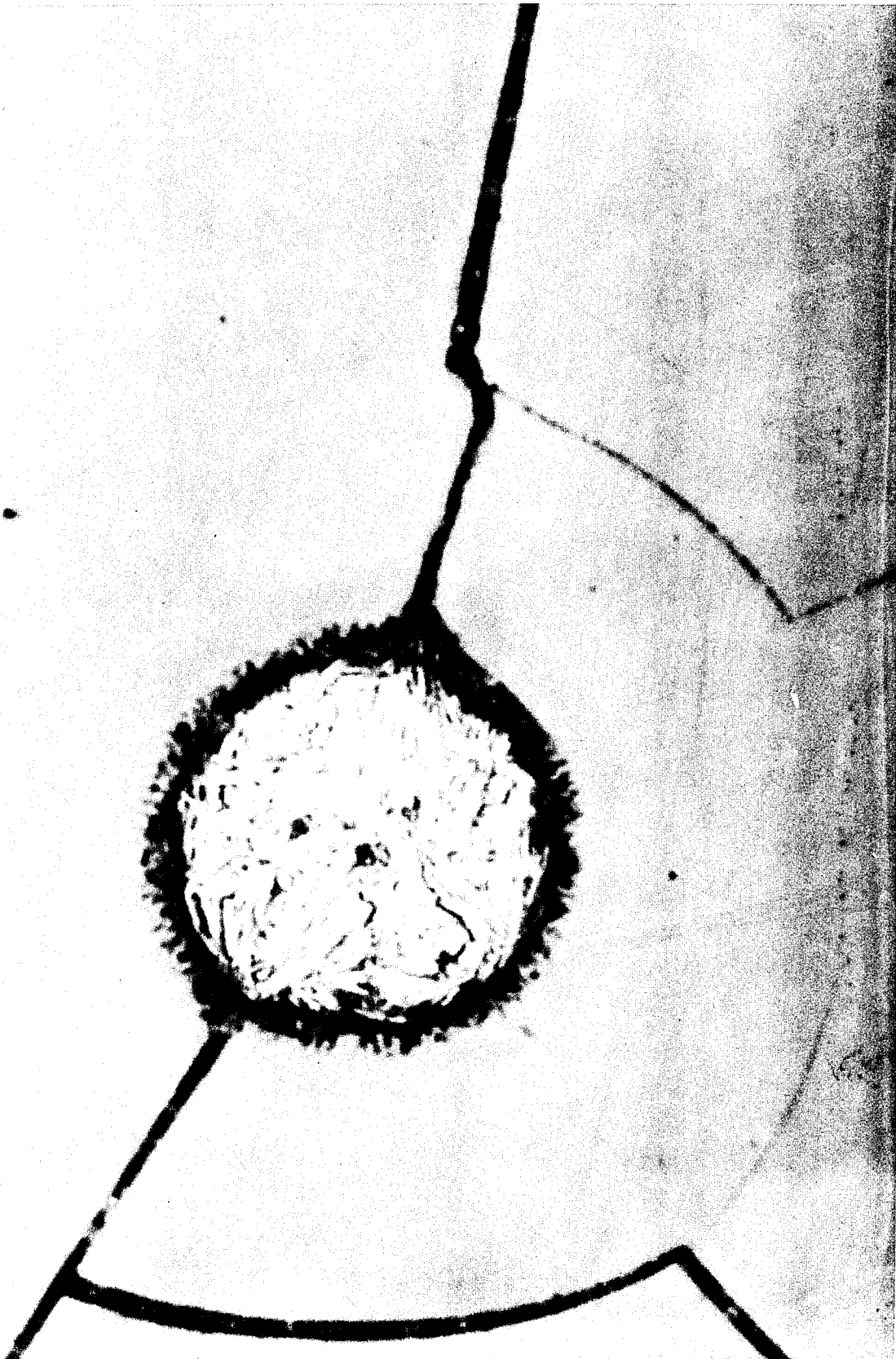
Fig. 22 - (2000X) View of core of damaged boron filament (BU #26) that has been etched to show evidence of melting
