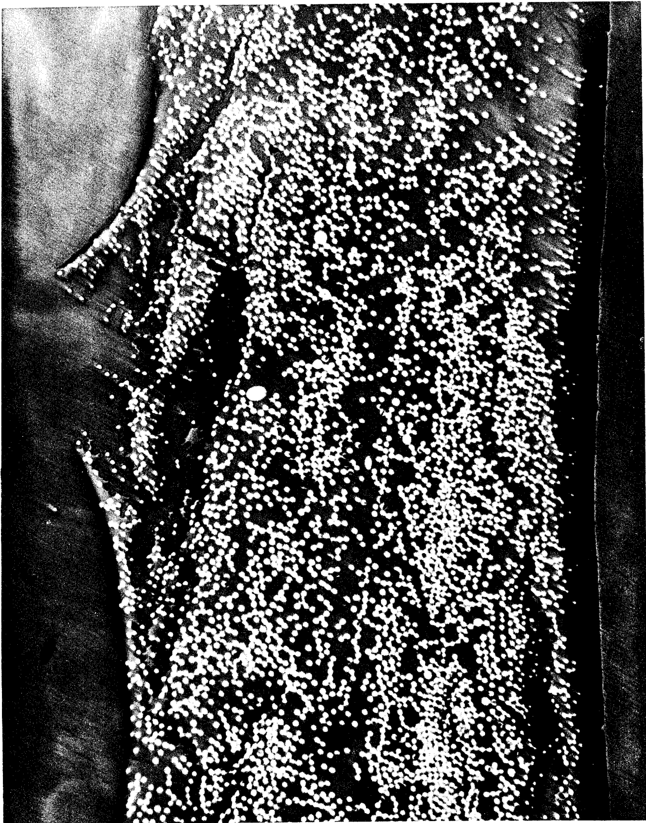
Fig. 37 - (100X) HM-S/epoxy specimen after 25 \times 10^4 amperes per \text{cm}^2 of filament crest current injection--some burning and delamination
