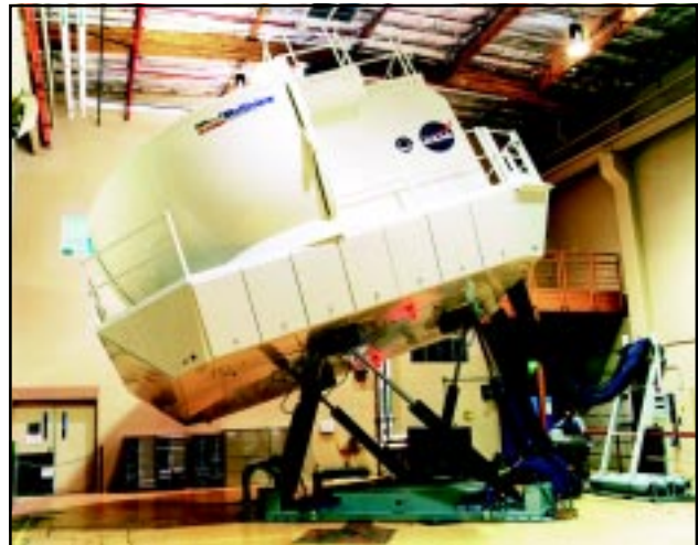
The new visual system is a wrap-around projector based system, which provides a cross-cockpit viewing capability and an enhanced field-of-view (40 degrees vertical by 180 degrees horizontal).
