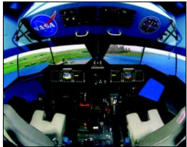
Interior view of the new TCAB with a Civil Tiltrotor out-the-window display.
