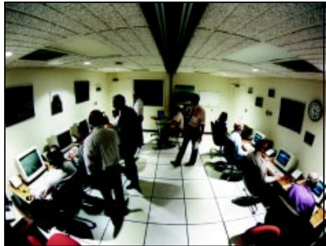
The Air Traffic Control (ATC) simulator was configured to use three of the four sector displays as “pilot” stations and one as an ATC Controller Station.
