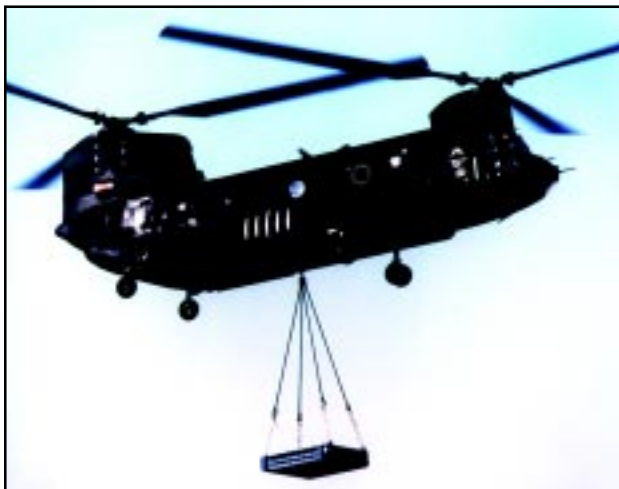
The Boeing CH-47D "Chinook" is the US Army's heavy cargo helicopter. There have been several modernization plans over the years which have been used to upgrade the aircraft.
