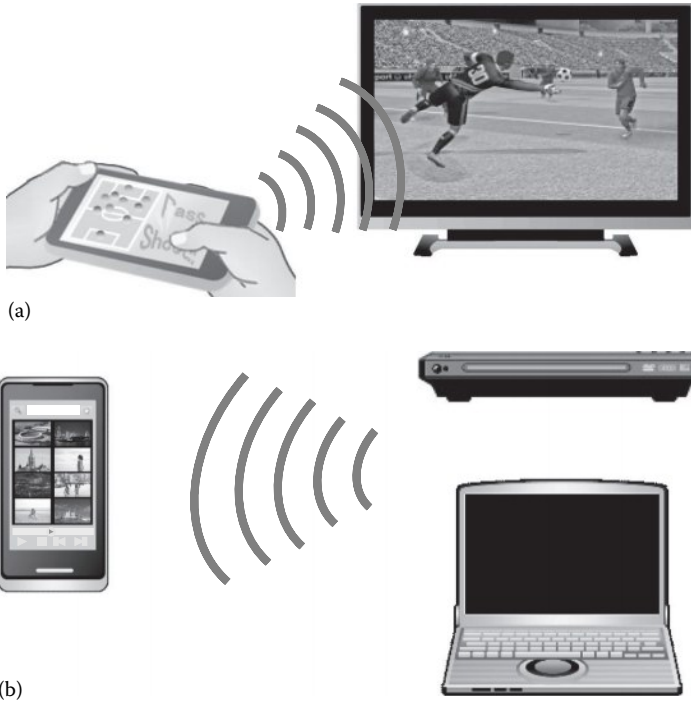
FIGURE 7.1 60 GHz mobile use case examples. (a) Low-latency video streaming and (b) fast file transfer.
