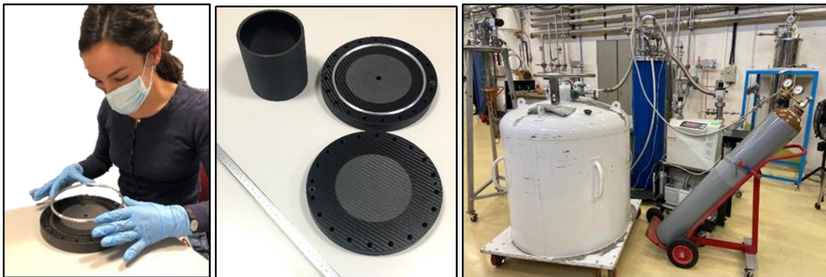
Fig.3 Pipe and flanges with special carbon materials and layup for leaktightness verification at cryogenic temperatures
