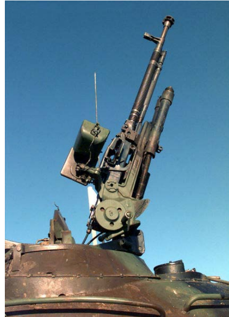
DShk 12.7mm Heavy Machine Gun, Bosnia, 1998 (Taken by DOD SSG Kim Price, Wikimedia Commons, August 2010)
