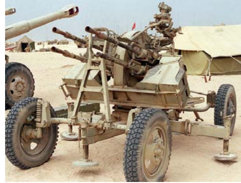
ZPU-4, Towed 14.5mm Anti-Aircraft Gun, Kuwait, 1991 (Taken by DOD LCPL Dunham, Wikimedia Commons, August 2010)
