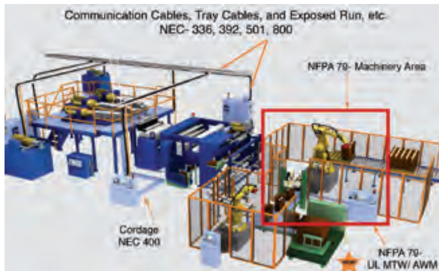
The diagram illustrates key NEC® and NFPA regulatory codes for an industrial plant manufacturing floor. Each code calls out permissible cables. 'NEC®' is a registered trademark of the National Fire Protection Association.
