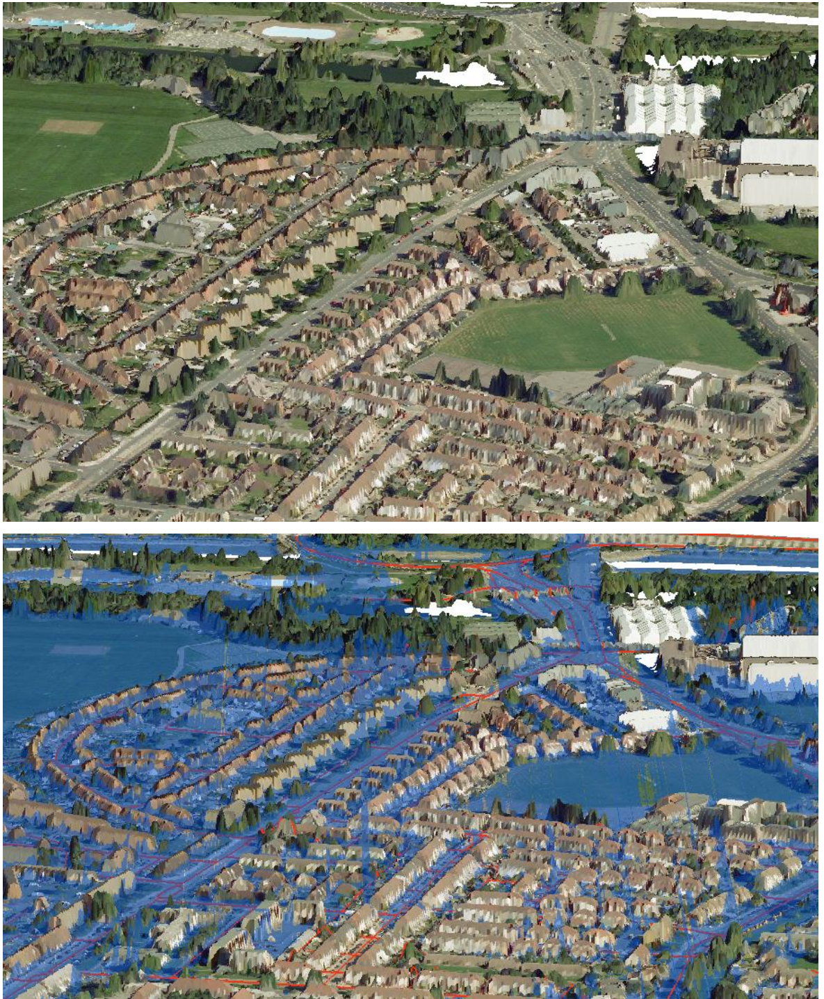
Figure 5.10. Zoomed in area of Hilsea aerial 3D hazard map; containing ortho-rectified aerial photo (OS), clipped Flood Zone 2 layer (blue shading) with added transparency and ITN (red lines) (Sources: Environment Agency, OS Mastermap Topography Layer & OS Aerial Imagery).
