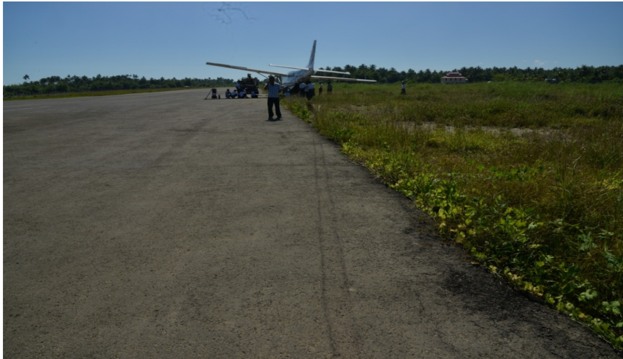
Figure :8 The Ground Mark of Right Main Wheel (Viewed from Runway-16 to Crash Site )
