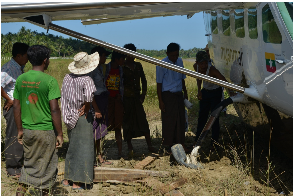
Figure :4 The Nose Wheel bobbed down with broken yoke
