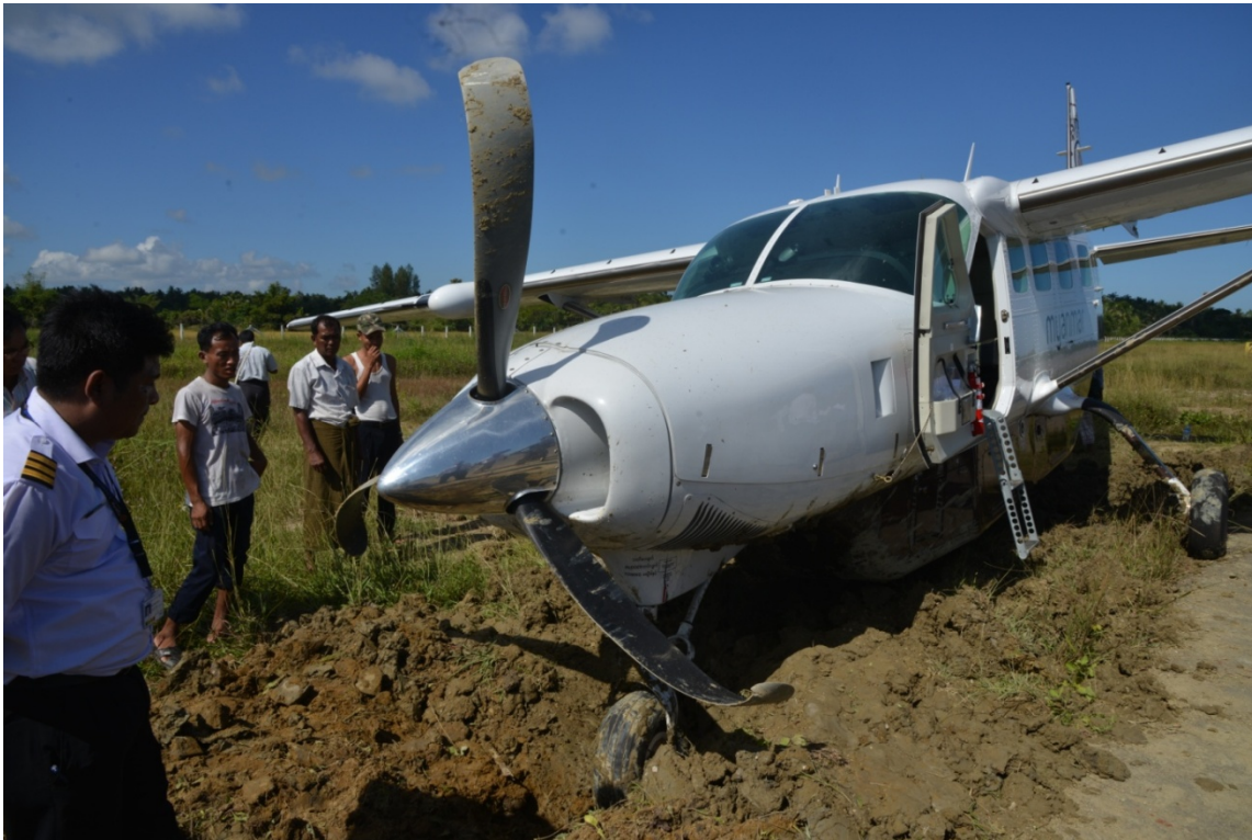
Figure:10 The twisted and damaged propeller
