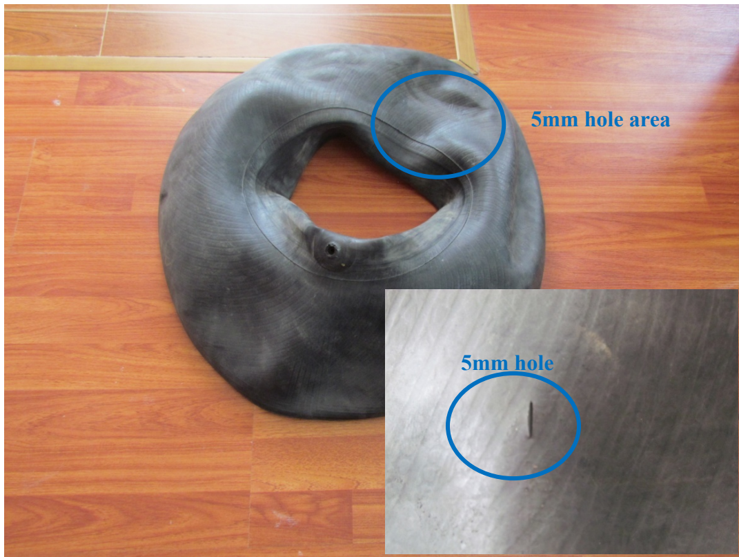
Figure:12 The 5mm hole and broken valve stem of the inner tube
