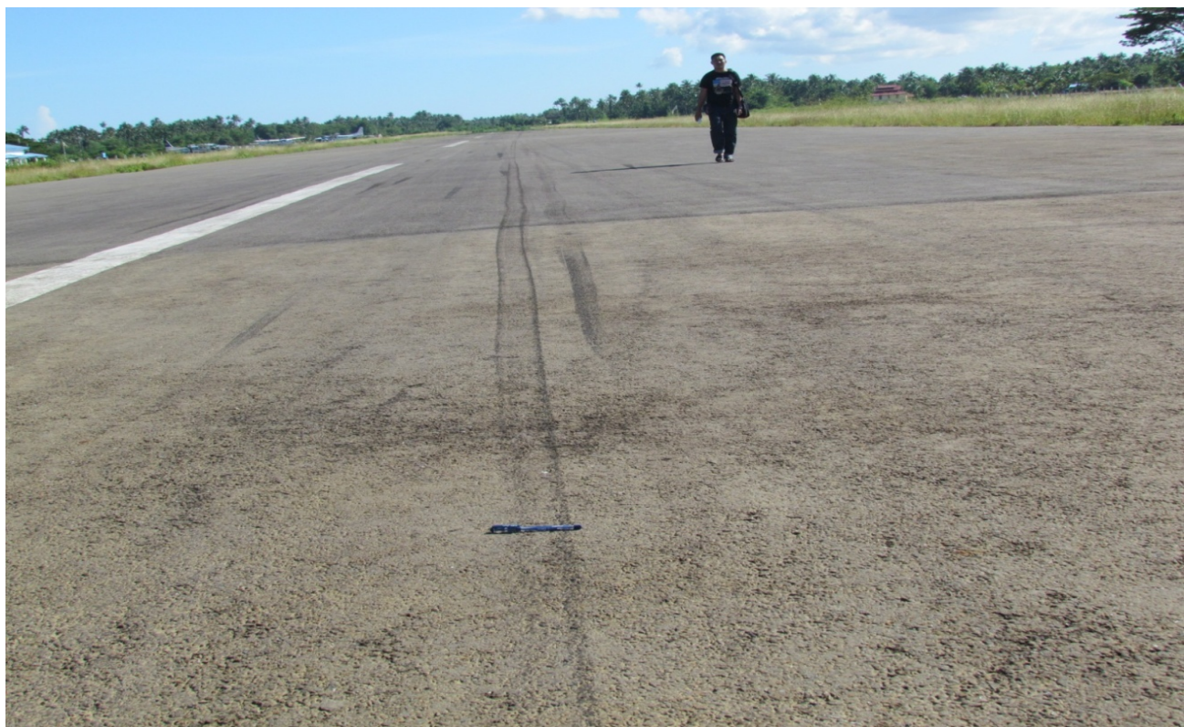
Figure:9 The Ground Mark of Right Hand Main Wheel (Viewed from Runway-16 to Crash Site )
