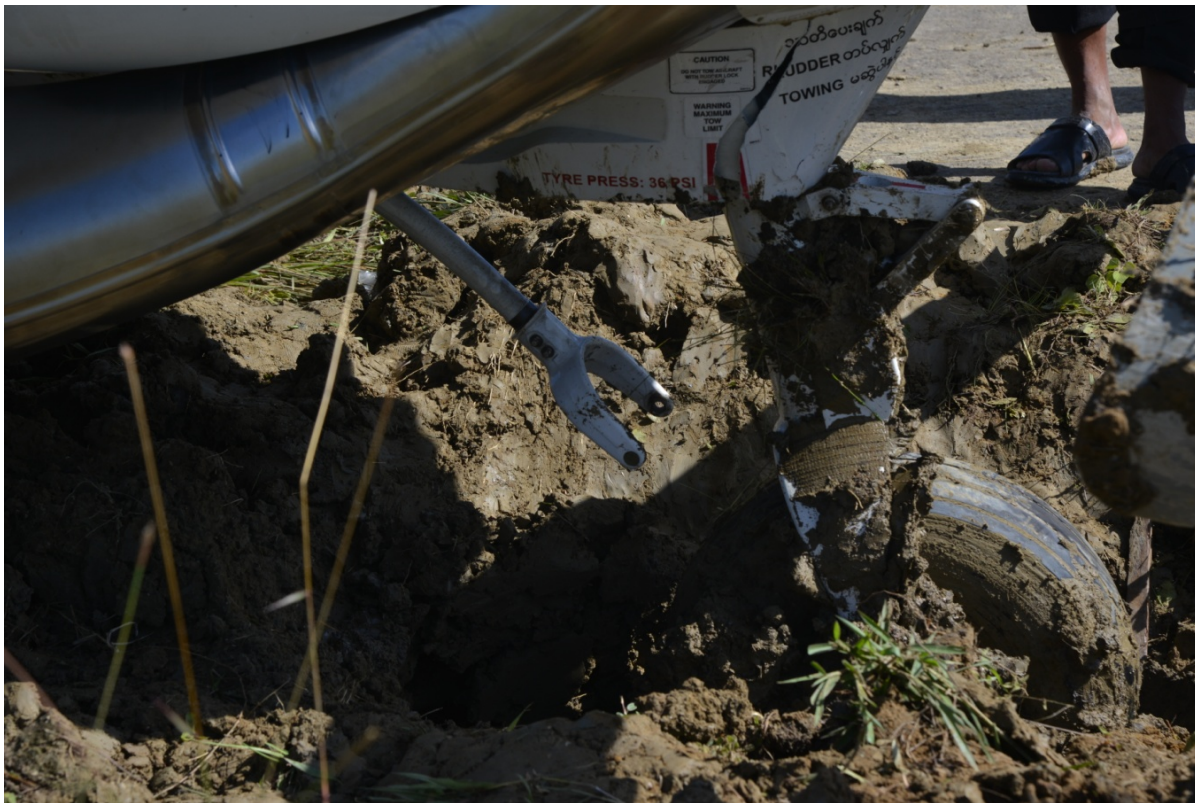
Figure :4 The Nose Wheel bobbed down with broken yoke
