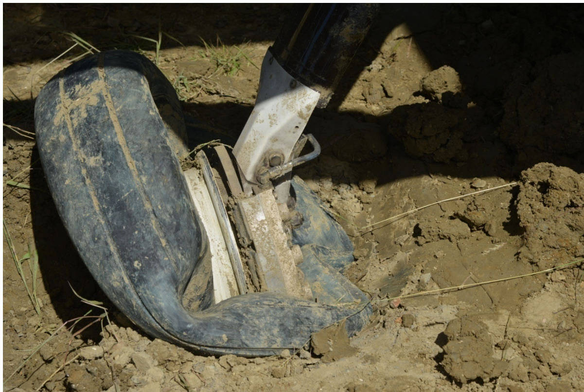
Figure :6 The Closer view of the damaged right hand Main Wheel
