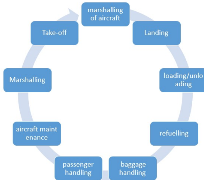
Figure 41: Cycle of ground handlers' support for aircrafts
