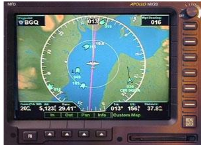
Figure 3: In this display, traffic can be seen superimposed on the surrounding terrain. The information is received live from other transmitting aircraft and from the ground-based transceiver.
