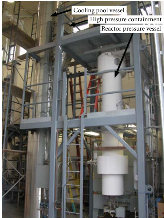
FIGURE 2: OSU-MASLWR experimental facility photo [1, 2, 13].
