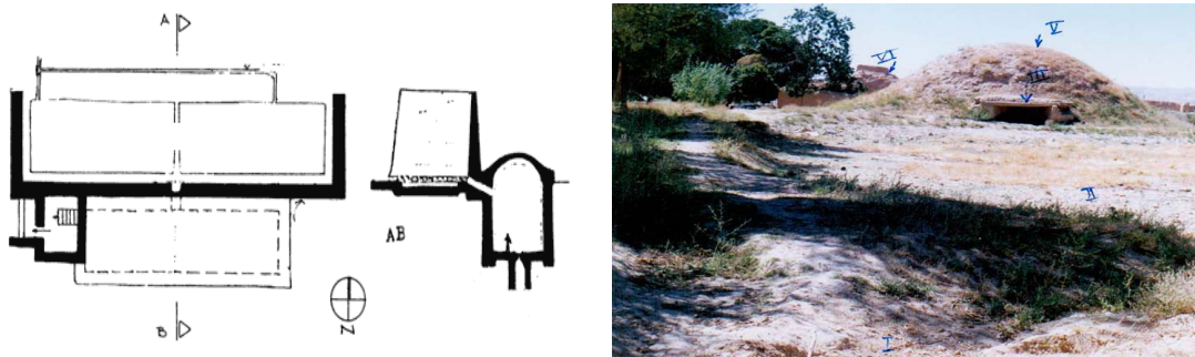
Figure 8. Different domed roof fridges in Iran (Ghobadian, 2007, p. 135)
