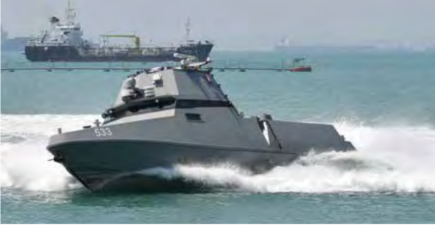
Singapore's MARSEC USV – a variant of the VENUS unmanned surface vehicle – is equipped with the autonomous Collision Detection' and Collision Avoidance (CDCA) system.
