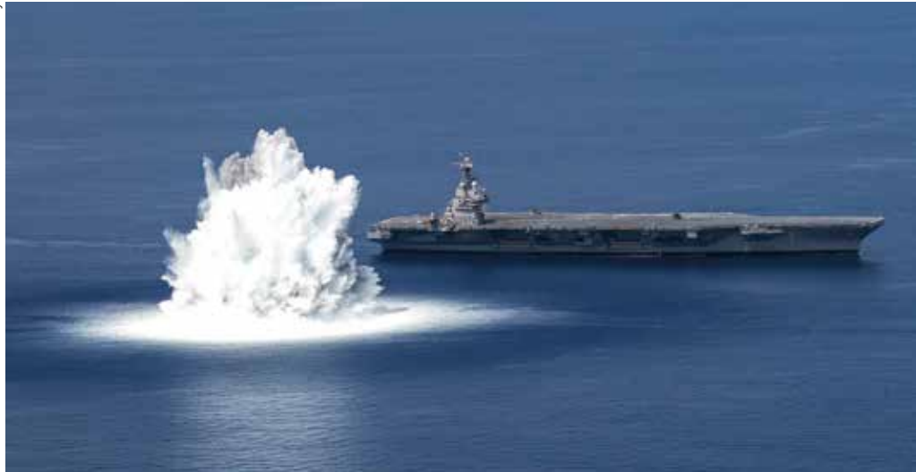
GERALD R. FORD (CVN-78) undergoing shock trials. The need to provide resistance against underwater shock has an important influence on warship habitability, impacting how cabins and passageways are designed.
