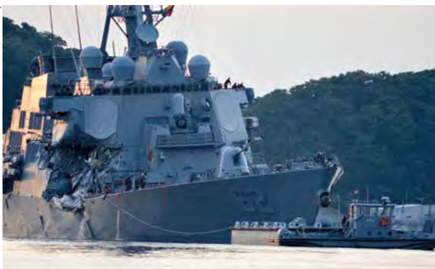
The US Navy destroyer FITZGERALD (DDG-62) being towed into port after her collision with the merchant vessel ACX CRYSTAL in June 2017.
