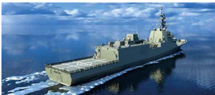
A concept image of the aft starboard view of the FFG-62 design. The hangar will accommodate one manned and one unmanned helicopter.
