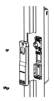
ENSURE that the lock is fully secured and flush to the mounting surface in order to depress tamper switch on back of device for correct operation.
