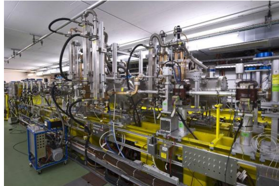
Two-beam test stand
