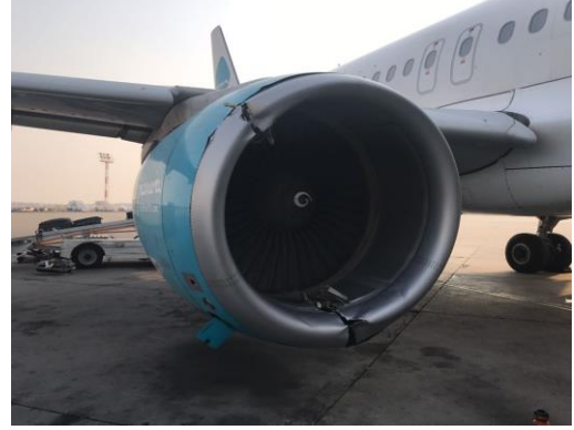
Figure 1. Engine inlet cowl damage
