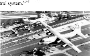
Using its aft loading ramp and door the C-130 can accommodate a wide variety of oversized cargo, including everything from utility helicopters and six wheeled armored vehicles to standard palletized cargo and military personnel. In an aerial delivery role, it can air drop loads up to 42,000 pounds or use its high-floatation landing gear to land and deliver cargo on rough, dirt strips.
