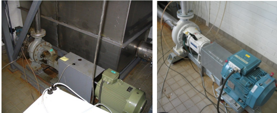
Fig. 4. Two laboratory pumping systems in the previous pump laboratory of Lappeenranta University of Technology. Serlachius pumping system on the left was acquired in 1970's and the Sulzer pumping system on the right in 2006.
