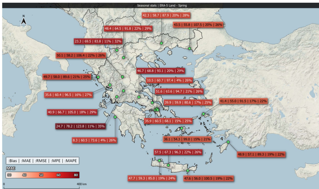
Figure 4. Bias ( W/m^2 ), MAE ( W/m^2 ), RMSE ( W/m^2 ), and MPE and MAPE (both ranging from 0 to 1 for better visualization) between ERA5-Land and surface observations for spring (MAM) in the Greek area.
