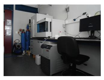
**Fig.1:** Inductively Coupled Plasma Mass Spectrometry (model iCAP-Qc)v
