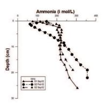
**Fig.4**: Porewater profiles of ammonia at stations S1 (September 2012) and S2 (February and September 2012)
