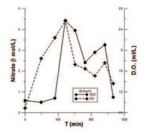
**Fig.6**: Dissolved oxygen and nitrate concentrations at station S2 during September 2012 (incubation of induced anoxia)
