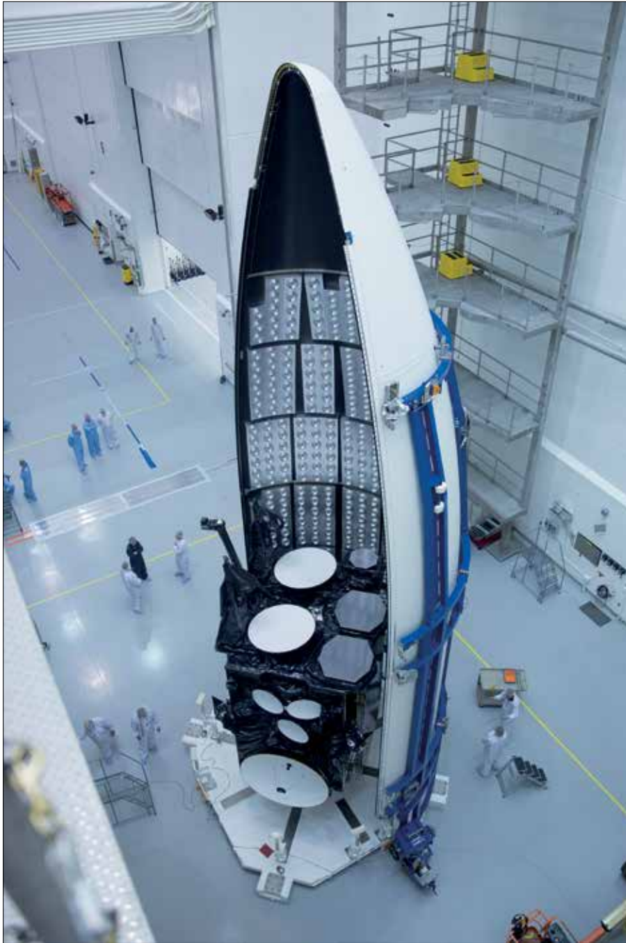
Workers prepare for launch of third Advanced Extremely High Frequency satellite, a joint-Service system that provides survivable, near worldwide, secure, protected, and jam-resistant communications for high-priority national military operations (Courtesy Lockheed Martin)
