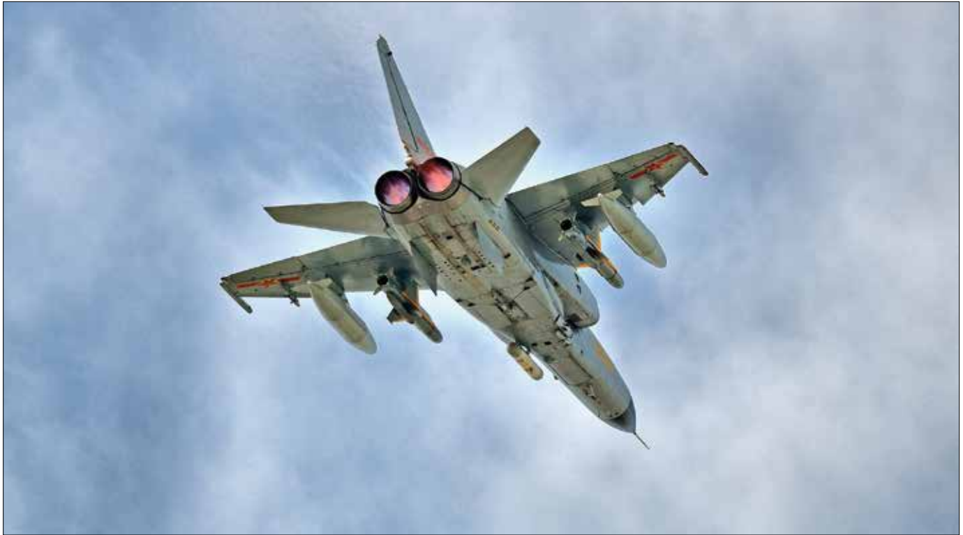
JH-7A fighter-bomber carrying KD-88 land-attack cruise missiles and drop tanks (Courtesy Sino Defense)
