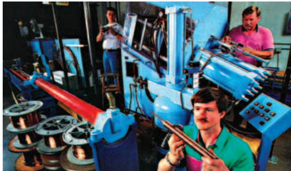
The Hydrostatic Extrusion Press: This apparatus makes complex structures into wires by pushing a complex array of copper, superconductor and strengthening material through a die at high pressure so that it all bonds together and can be made into long wires suitable for making magnets. Pictured, from left, are: Rob Heussner (a former Applied Superconductivity Center graduate student); Bill Starch, the APC lab manager who is among those making the move to FSU; and Paul Jablonski (a former APC graduate student).
