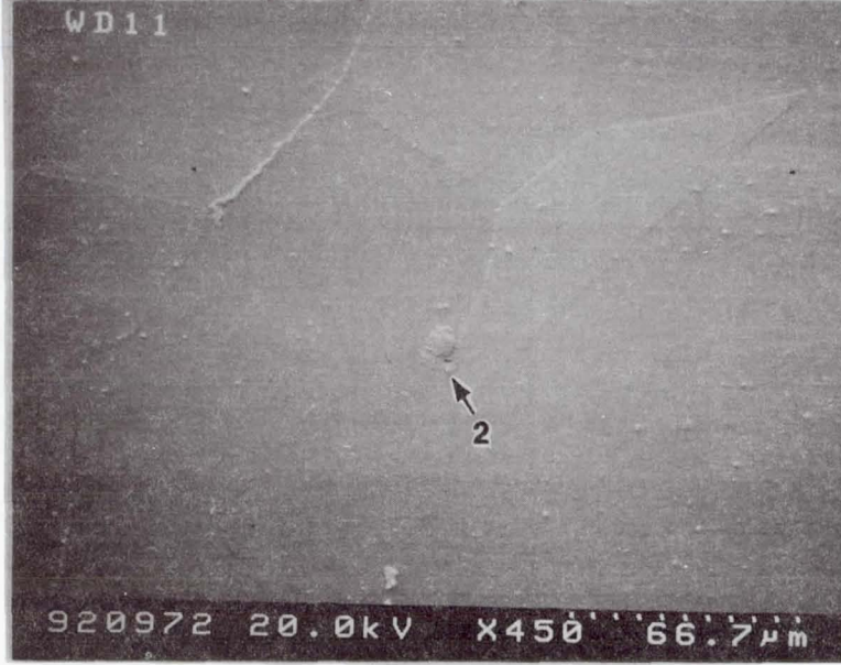
Figure 13. Optical (a) and SEM (b, c, d) micrographs after sample was exposed at 970 °C (1,780 °F) for 6 h, showing islands and incipient melting. Arrows represent same area.
