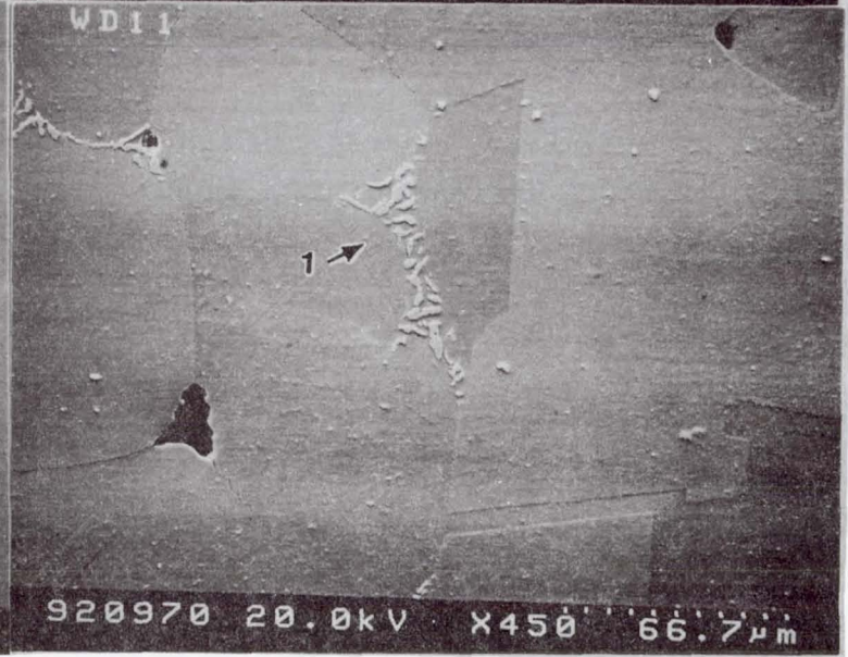
Figure 13. Optical (a) and SEM (b, c, d) micrographs after sample was exposed at 970 °C (1,780 °F) for 6 h, showing islands and incipient melting. Arrows represent same area.
