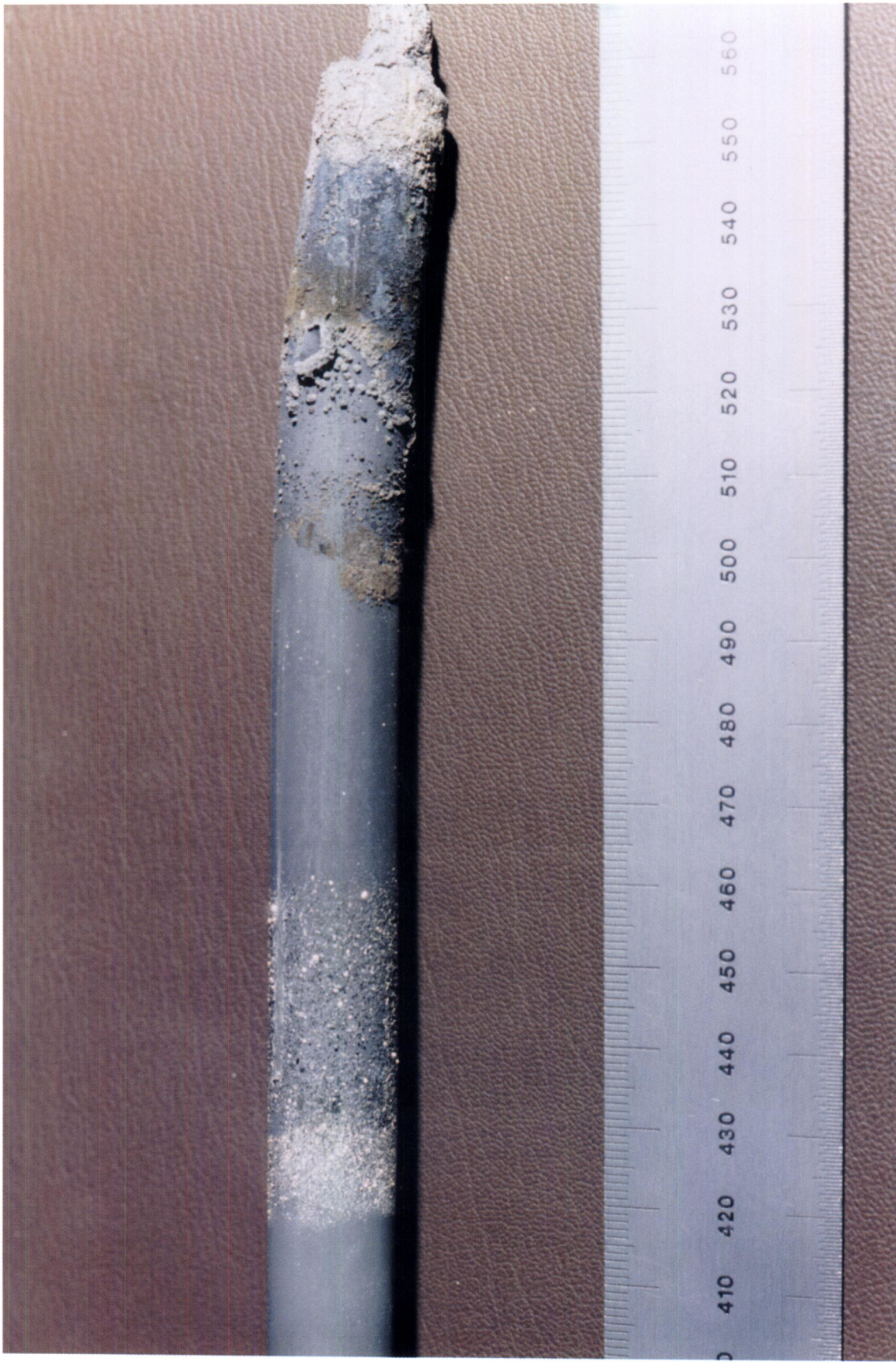
Figure 10.7 Flight cartridge, post-mission showing severe bending Scale is in cm.
