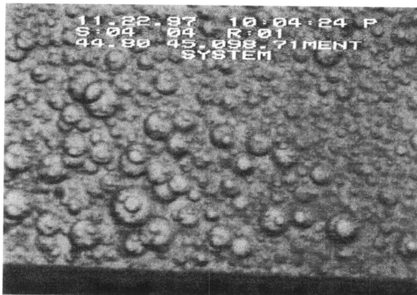
Figure 5. Image obtained from a 55 wt% GLY sample during processing. The gasket material is seen at the bottom of the image and the succinonitrile-glycerol mixture is at the top.
