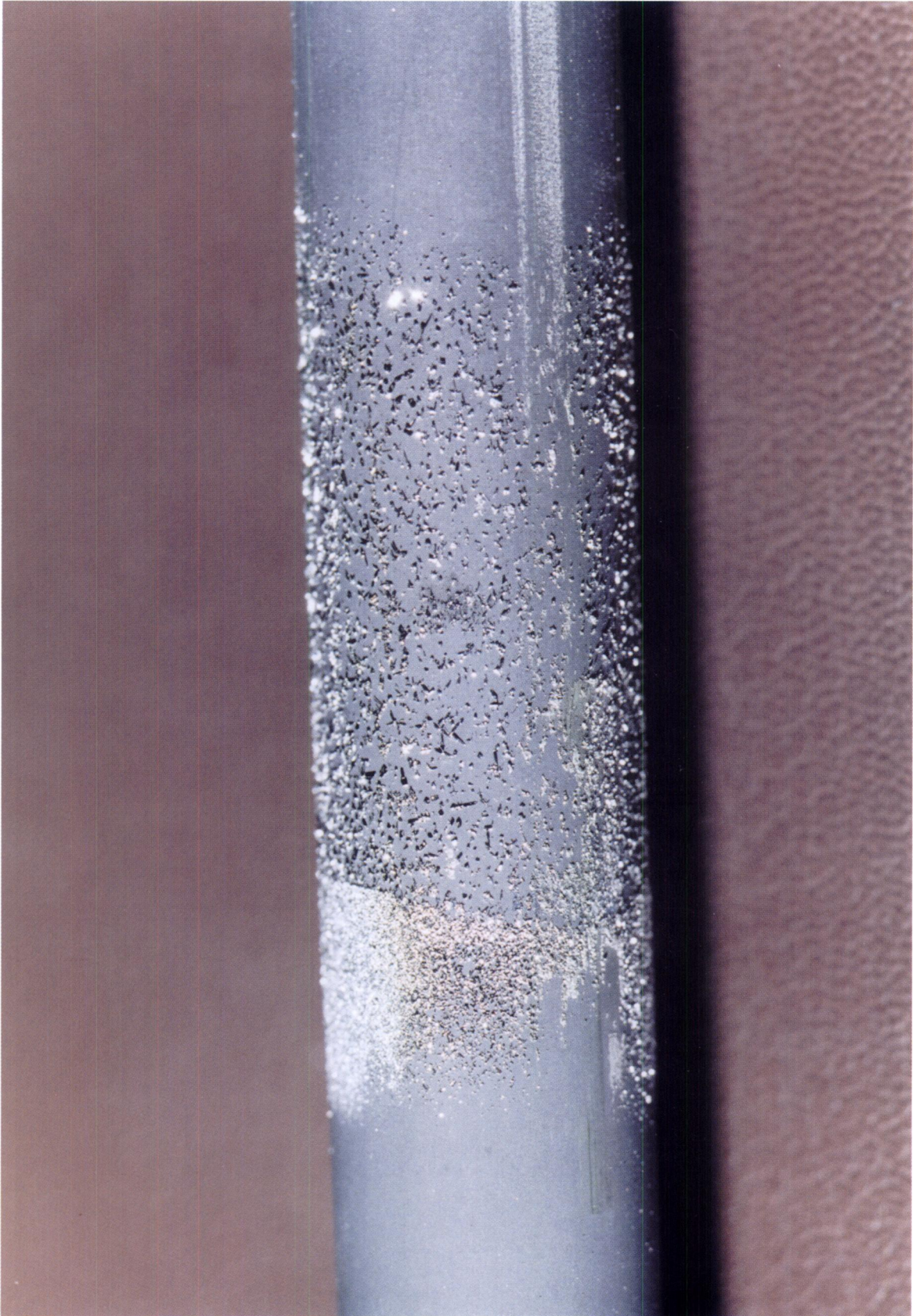
Figure 10.8 Close up of crystalline deposits on surface of cartridge SL1-417
