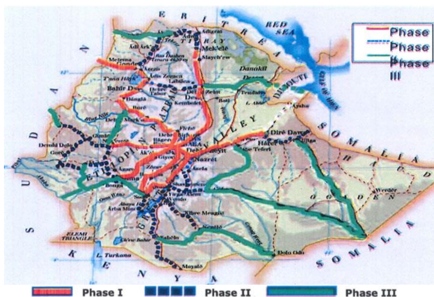
Source : Ministry of Communication and Information Technology (MCIT), Ethiopia Figure 5.5.2 Development plan of backbone optical fiber network (2012)
