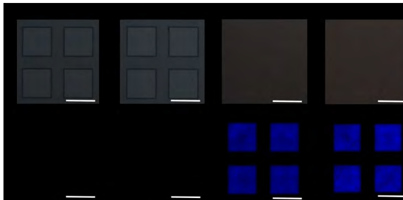
Micrographs of mechanophore-anchored polymer films on a silica substrate after laser impingement (a) 120 MPa. (b) 141 MPa. (c) 163 MPa, (d) 185 MPa. Scale bar 70 microns.
