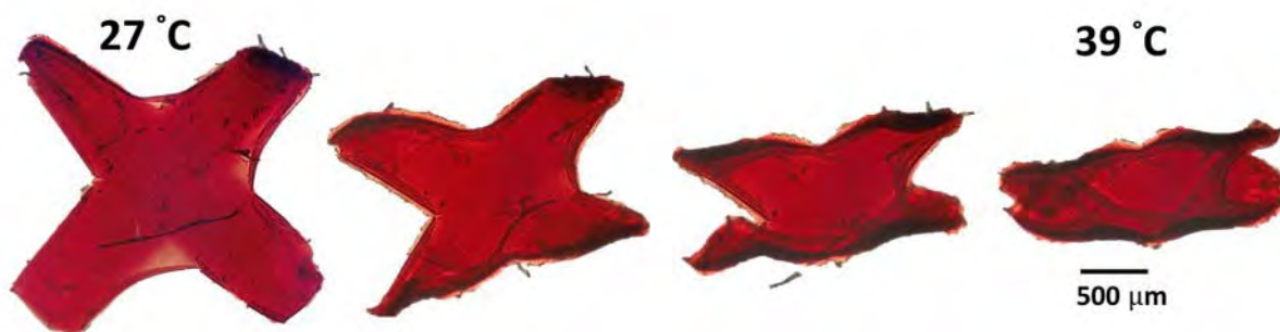
Figure 1: Reversible, 3D shape changes of the chromonic hydrogel with temperature
