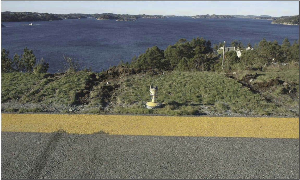
Figure 21: The end of the runway with skid marks left by the tyres. The nose landing gear on the left, followed by the left main landing gear, which left black stripes on the paved surface, and, to the far right at the edge of the photo, the skid mark left by the right main landing gear.
