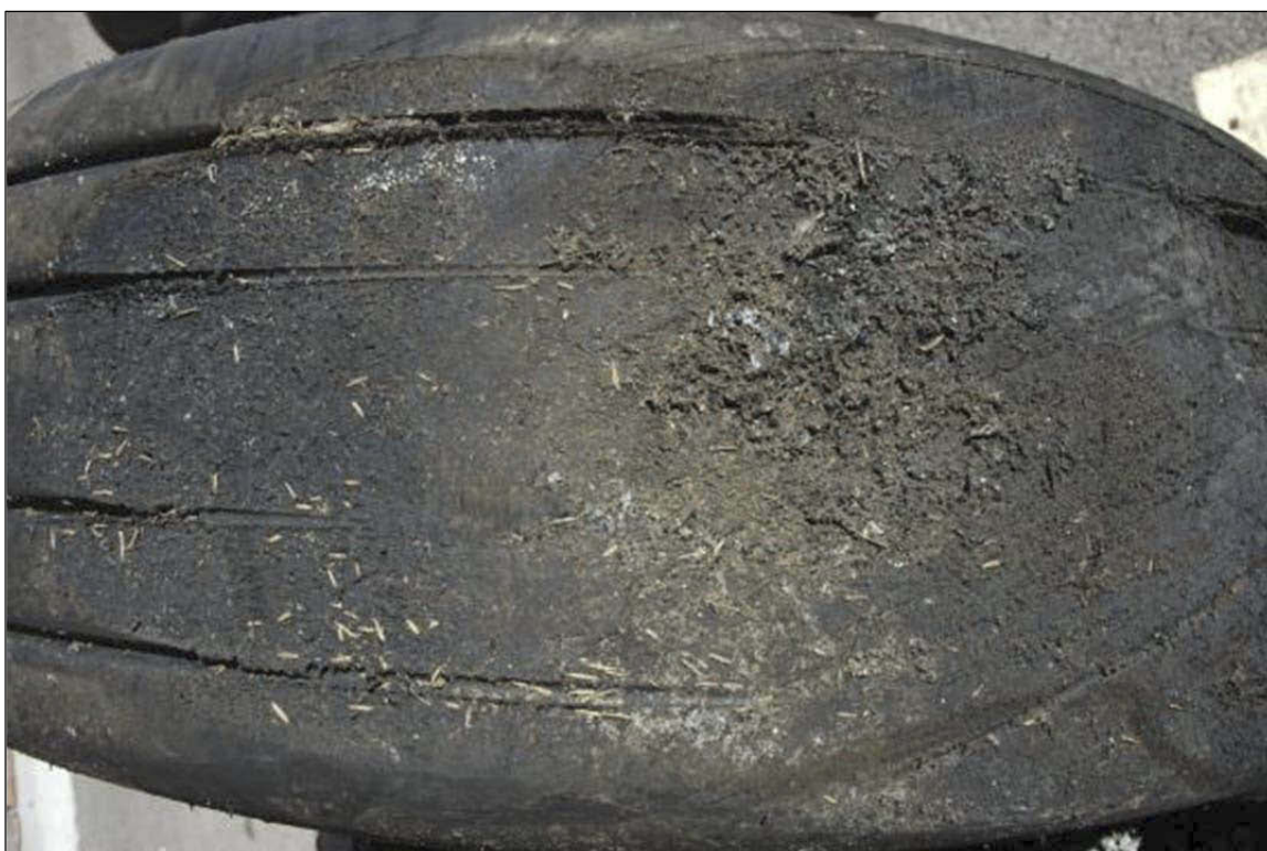
Figure 27: Wear marks on the left tyre of the left main landing gear. The tyre had moved from left to right at an angle of 27° in relation to the asphalt, for an unspecified period. Clumps of decomposed rubber on the right in the photo.
