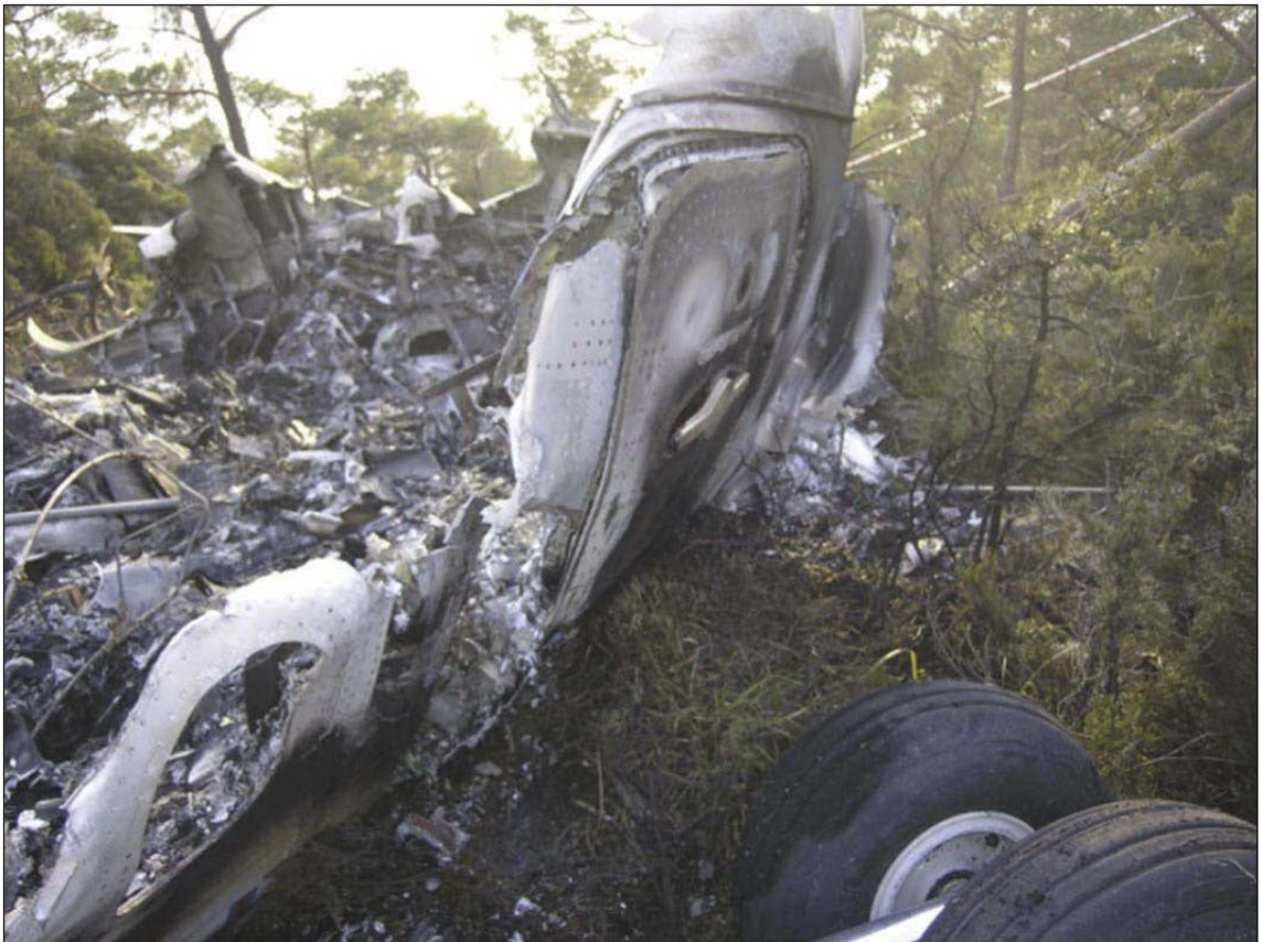
Figure 33: The cockpit and the blocked front right emergency exit. The door handle has been pushed out (partially opened). The nose wheels can be seen in the foreground on the right.
