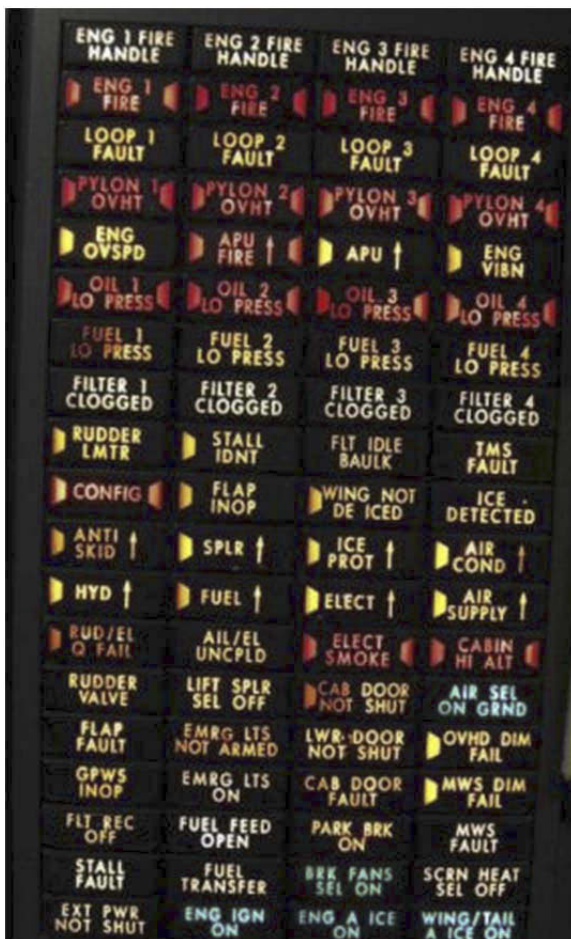
Figure 12: Master warning panel.
