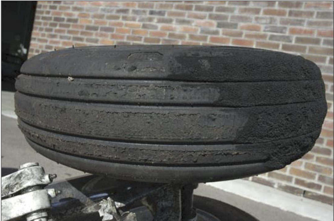
Figure 25: Right nose wheel. Clear wear marks on the left and heat damage on the right.
