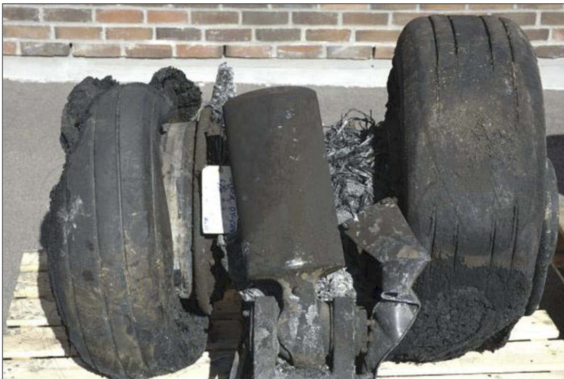
Figure 26: The wheels on the left main landing gear. The left wheel is on the right in the photo.
