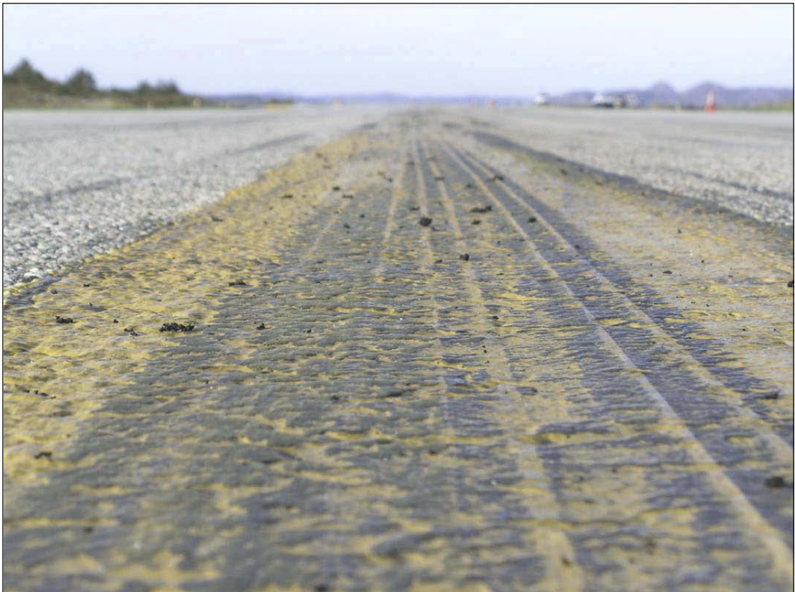
Figure 22: Close-up of small bits of rubber that were spread across the runway on both sides of the skid marks left by OY-CRG. (The black skid marks on the yellow runway markings are not from the aircraft involved in the accident).
