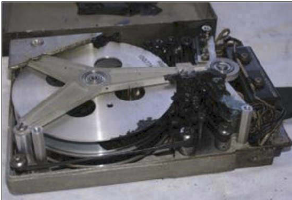
Figure 16: Heat-damaged storage unit in FDR.
