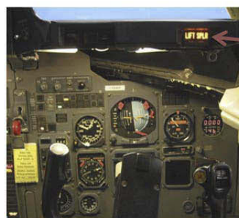
Figure 8: Glareshield lift spoiler light.
