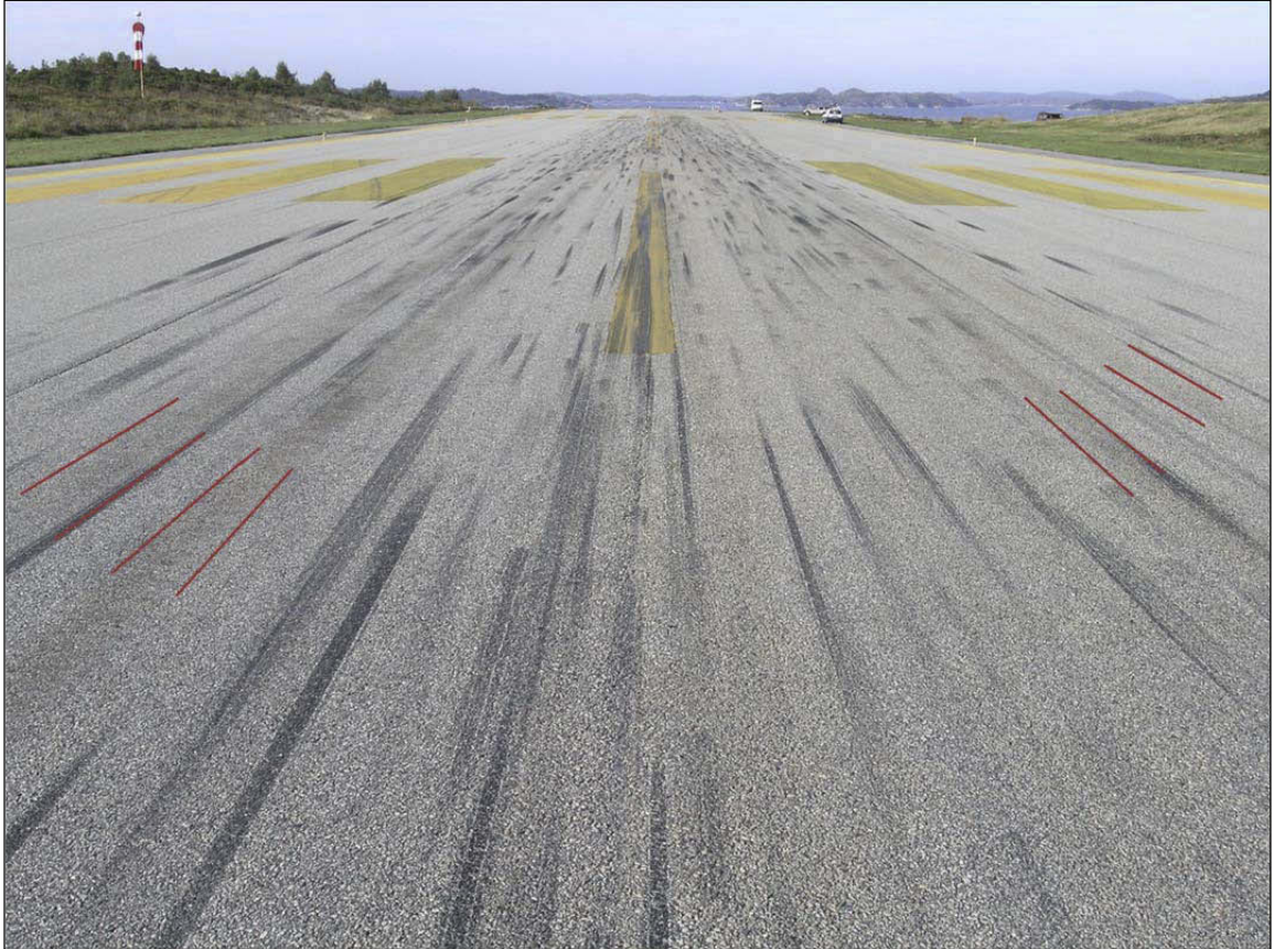
Figure 20: The skid marks left by OY-CRG on the runway. The red guiding lines show what route the main wheels took.
