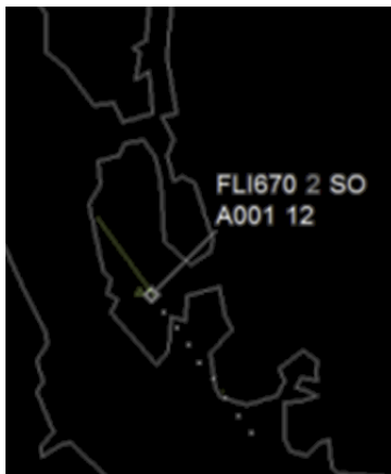
Figure 14: Shows FLI670 (OY-CRG) as it passed the threshold for runway 33. Ground speed: 120 kt.
