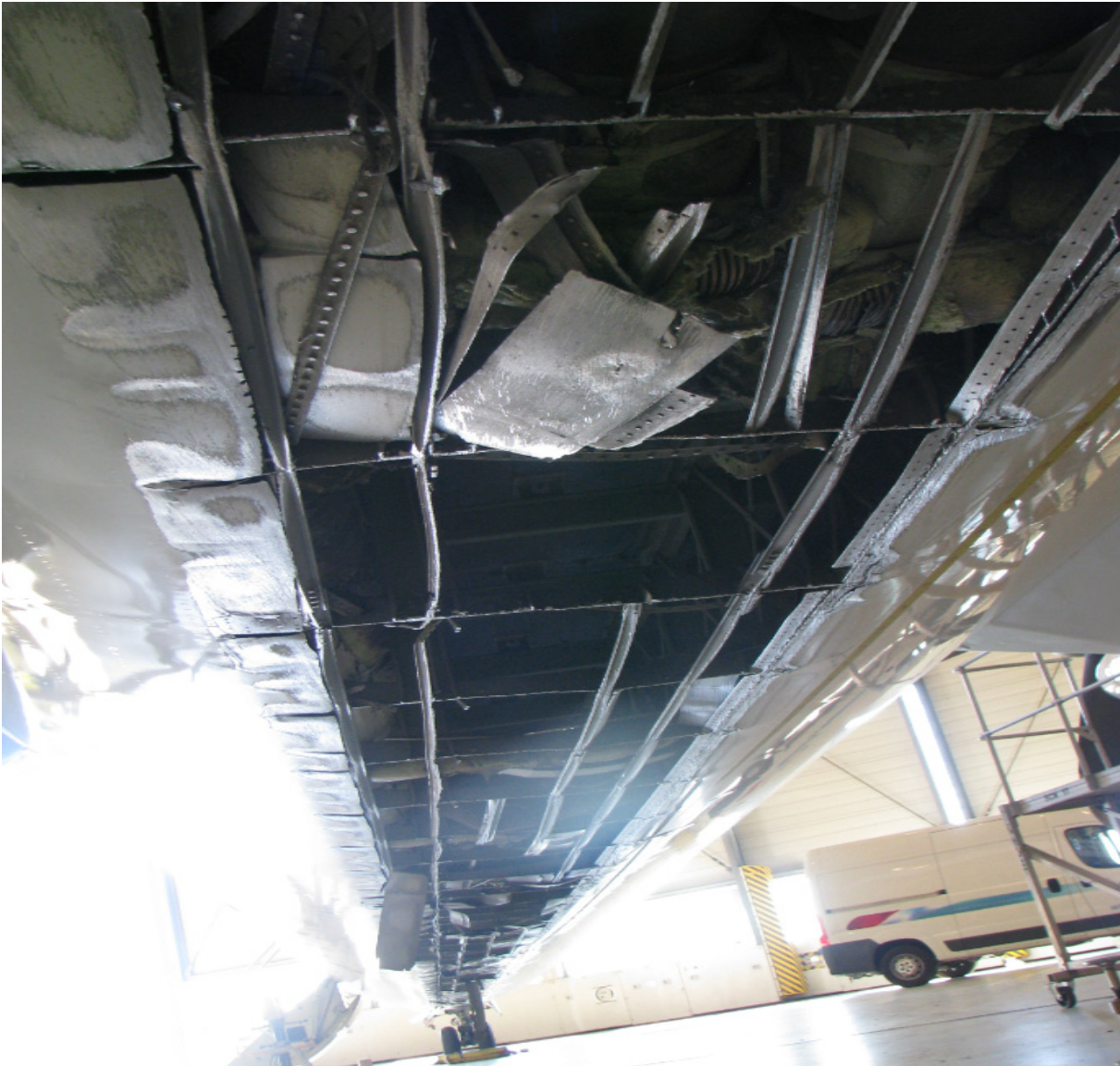
Damage on the fuselage's bottom surface (in flight direction)
