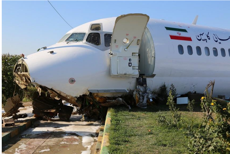
Figure 13- Damage to the fuselage nose
