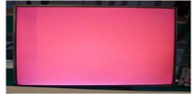
Vertical Block Source TAB IC Defect
