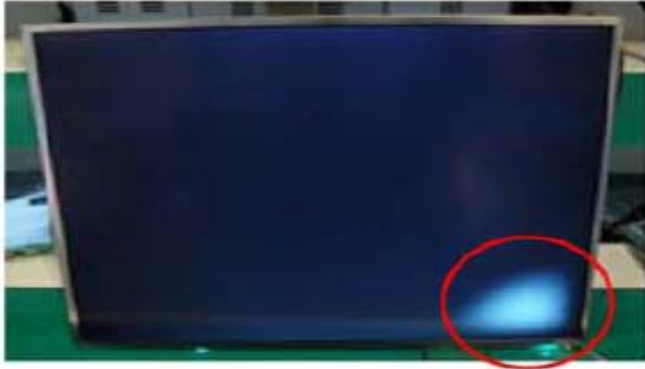
Panel Mura, Light leakage
