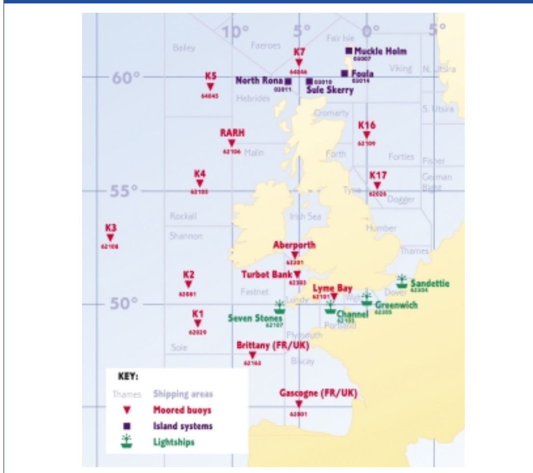
Figure 11: The UK Met Office Marine Automatic Weather Station Network, showing the locations of moored buoys around the UK
