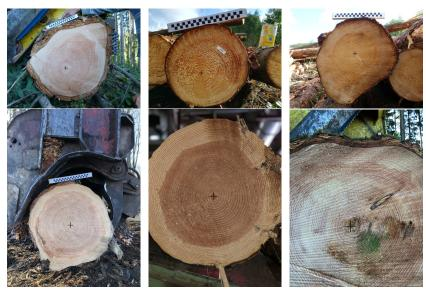
Fig. 5: Pith position (black cross) detected by the proposed method on raw log-end images using default parameters.
