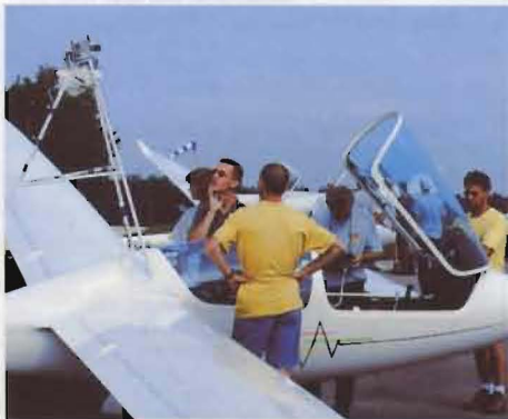
'Eiffel Tower' laser measures wing-bending on ASH-25
