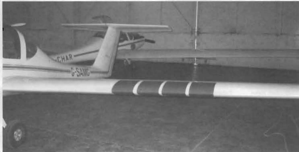
Despite fluorescent flashes on Grob G-109's wings, test pilots were unable to see the motorglider on some runs
