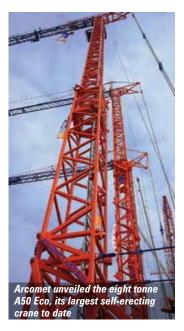
largest self-erecting crane to date, with a 50 metre jib with a jib tip capacity of 1,500kg. Jibs of 29, 35, 40 and 45 metres are also possible and hook heights range from 18.4 metres to 36 metres. The maximum counterweight is 42 tonnes with a tail swing/slew radius of 3.85 metres and a base footprint of 4.8 by 4.8 metres.
