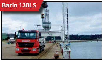
Total weight **17,500kg**Vertical reach below bridge deck **7.4m**Horizontal reach under bridge deck **13.00m**Platform payload **500kg**Width taken up on bridge deck **2.5m**Underbridge platform rotation **180 degrees**
